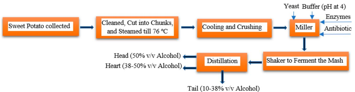
Figure 4. Scheme for the synthesis of bioethanol from sweet potato waste.
