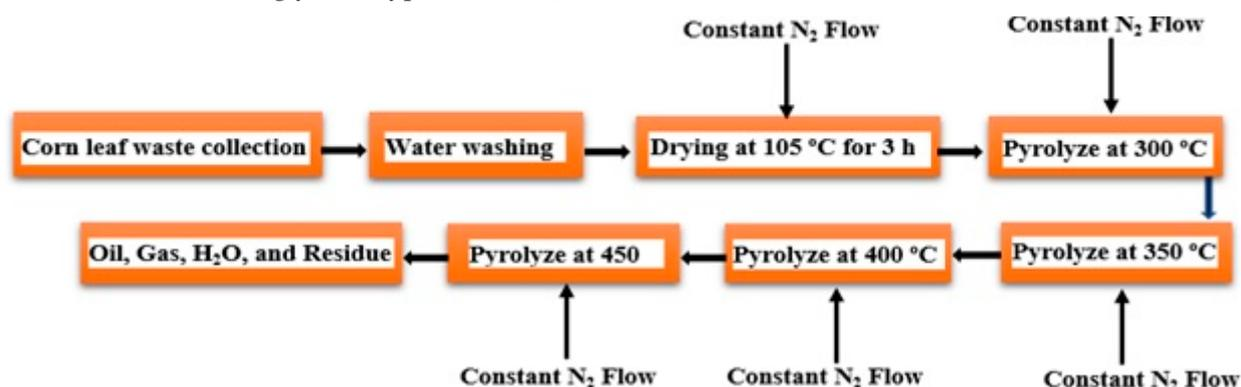
Figure 9. Scheme describing the synthesis of biofuel from corn leaf waste.
