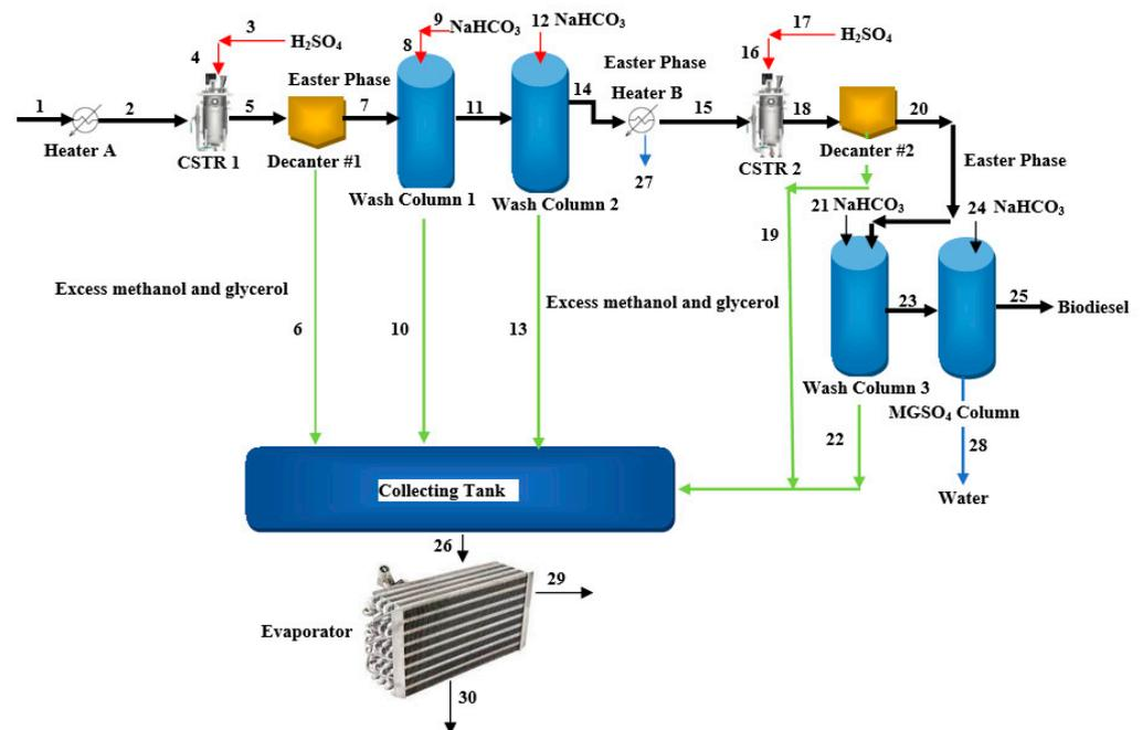
Figure 10. Process flow diagram for the synthesis of biodiesel from Jojoba seed oil.
