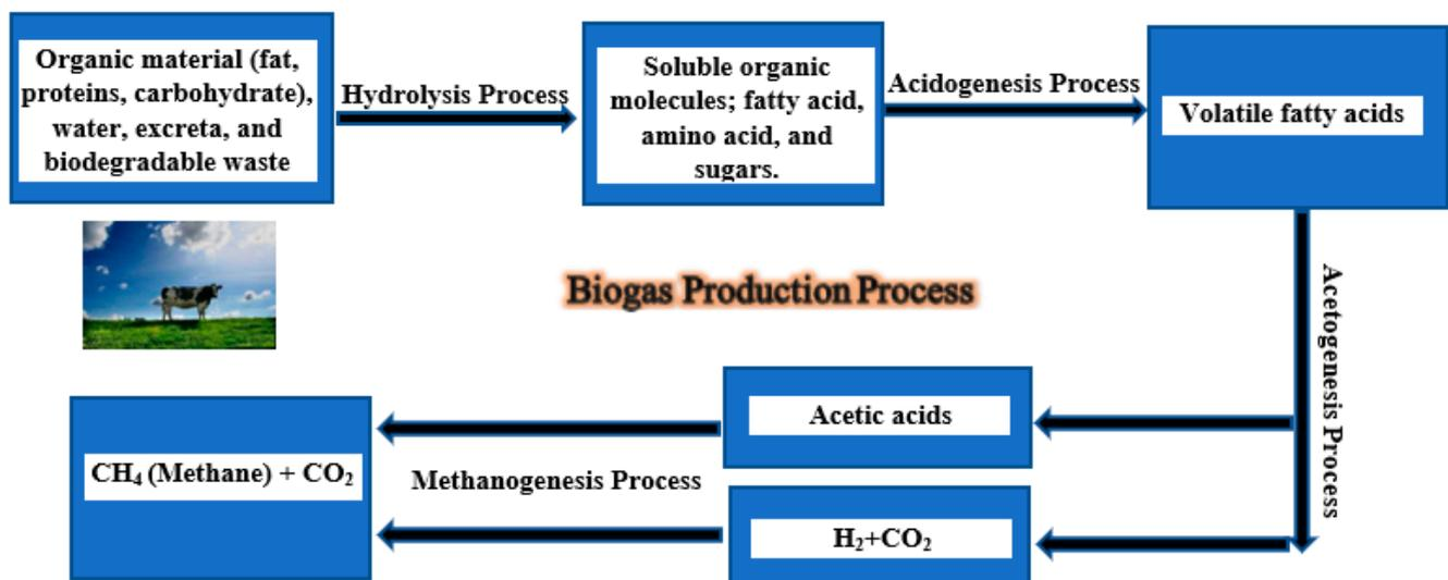
Figure 13. Scheme describing the production of biogas.
