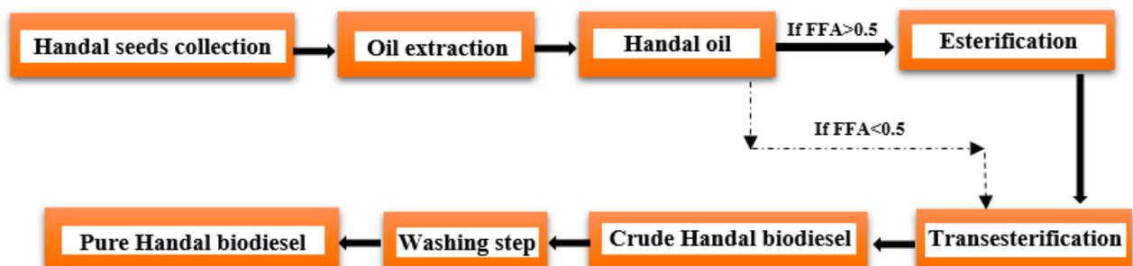
Figure 11. Process flow diagram for the synthesis of biodiesel from Handal seed oil.
