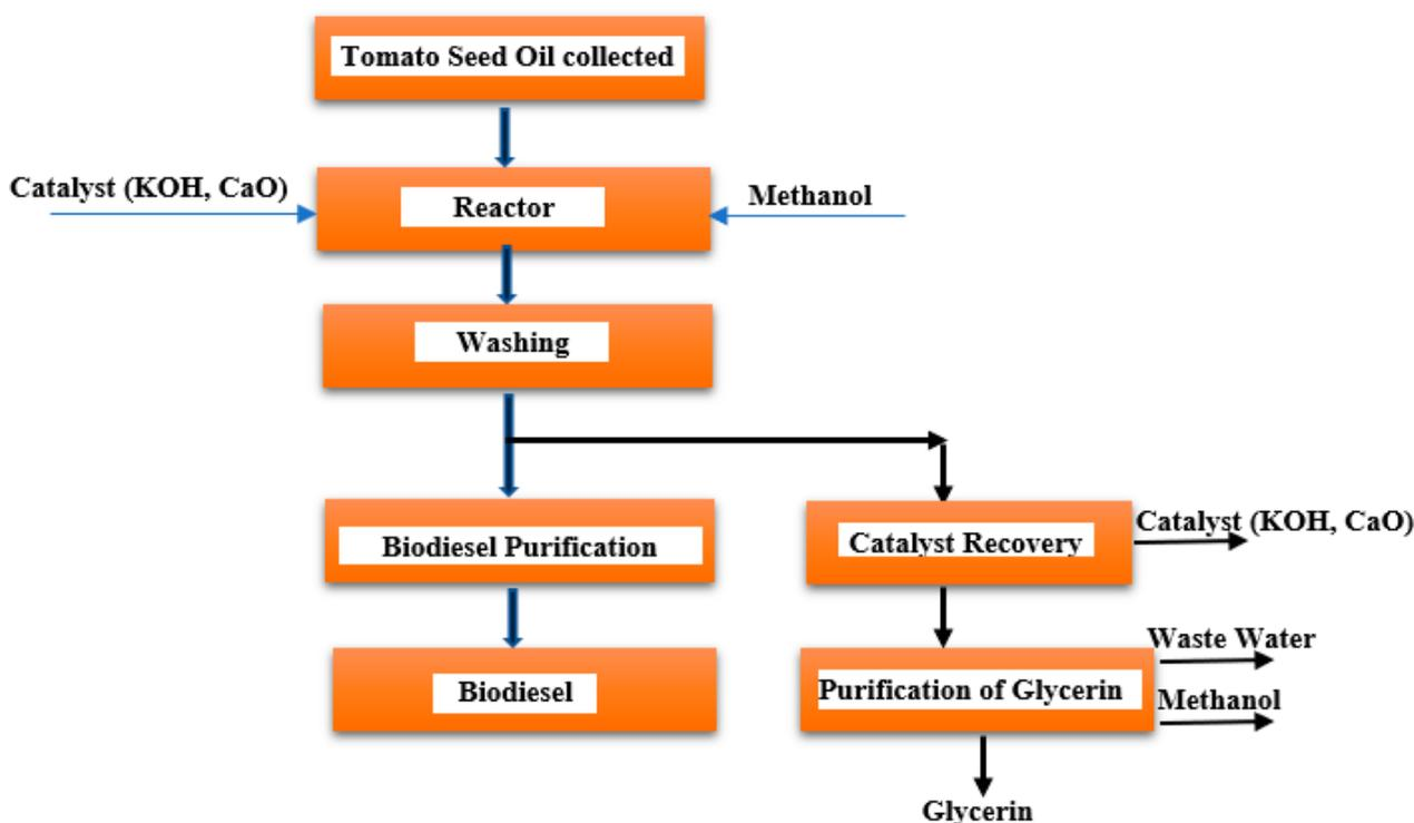
Figure 5. Scheme of the synthesis of biodiesel from tomato seed oil.
