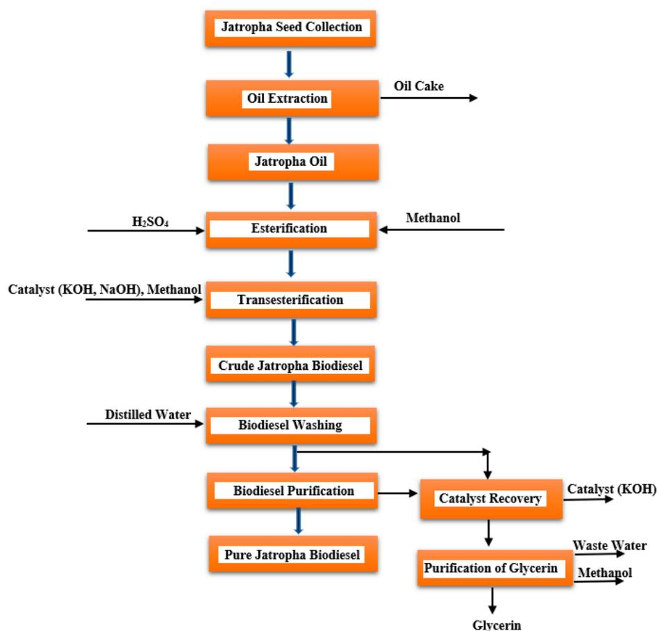
Figure 12. Process flow diagram for the synthesis of biodiesel from Jatropha seed oils.
