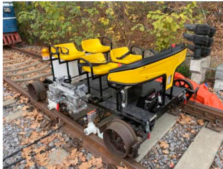
Figure 1. Physical picture of double-track rail flaw detection vehicle.
