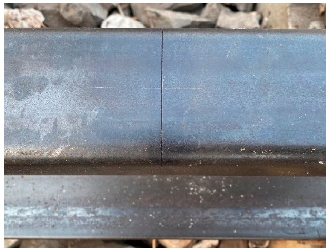
Figure 11. Example of artificial defect of rail.
