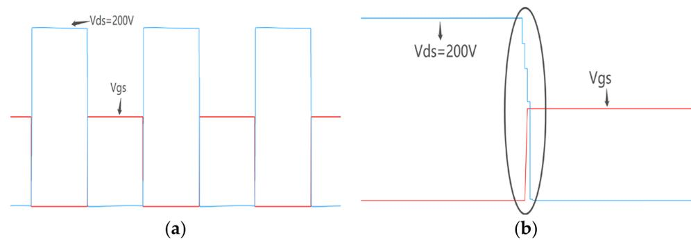
**Figure 8.** Simulation results for  $f_s = 140$  kHz: (a) Steady-state waveforms (time scale:  $4 \mu\text{s}/\text{div}$ ); (b) partial amplification waveforms (time scale:  $800 \text{ ns}/\text{div}$ ).
