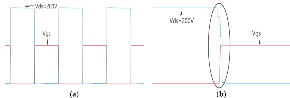
**Figure 7.** Simulation results for  $f_s = 125$  kHz: (a) Steady-state waveforms (time scale: 4  $\mu$ s/div); (b) partial amplification waveforms (time scale: 800 ns/div).
