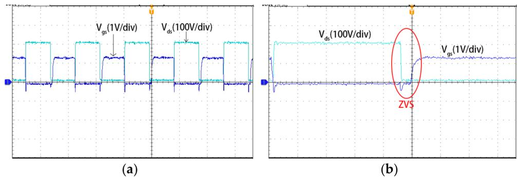
**Figure 11.** Experimental results for  $f_s = 140$  kHz: (a) Steady-state waveforms (time scale:  $4 \mu\text{s}/\text{div}$ ); (b) Soft-switching waveforms (time scale:  $800 \text{ ns}/\text{div}$ ).
