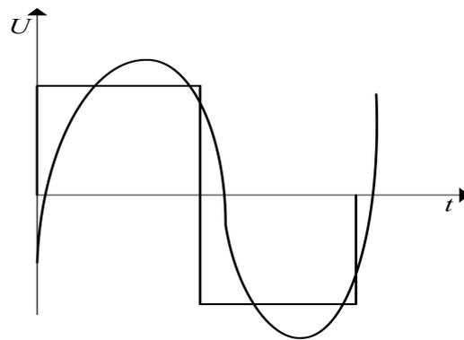
Figure 4. The working waveform of the full-bridge LLC resonant converter.
