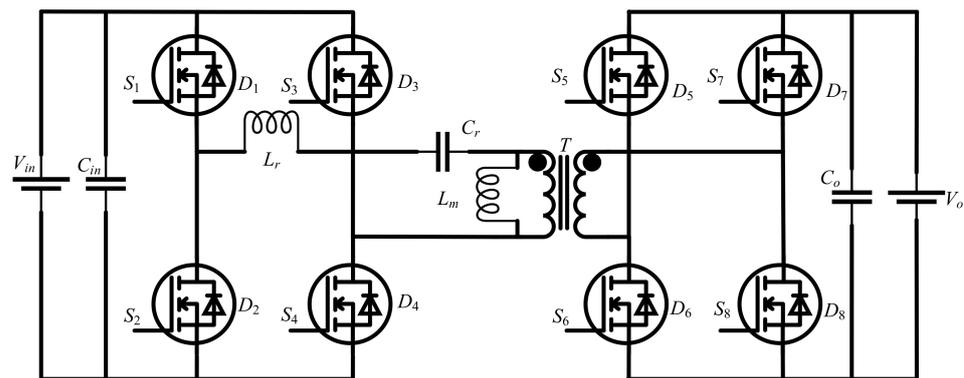
**Figure 1.** The topology of the full-bridge LLC resonant converter.
