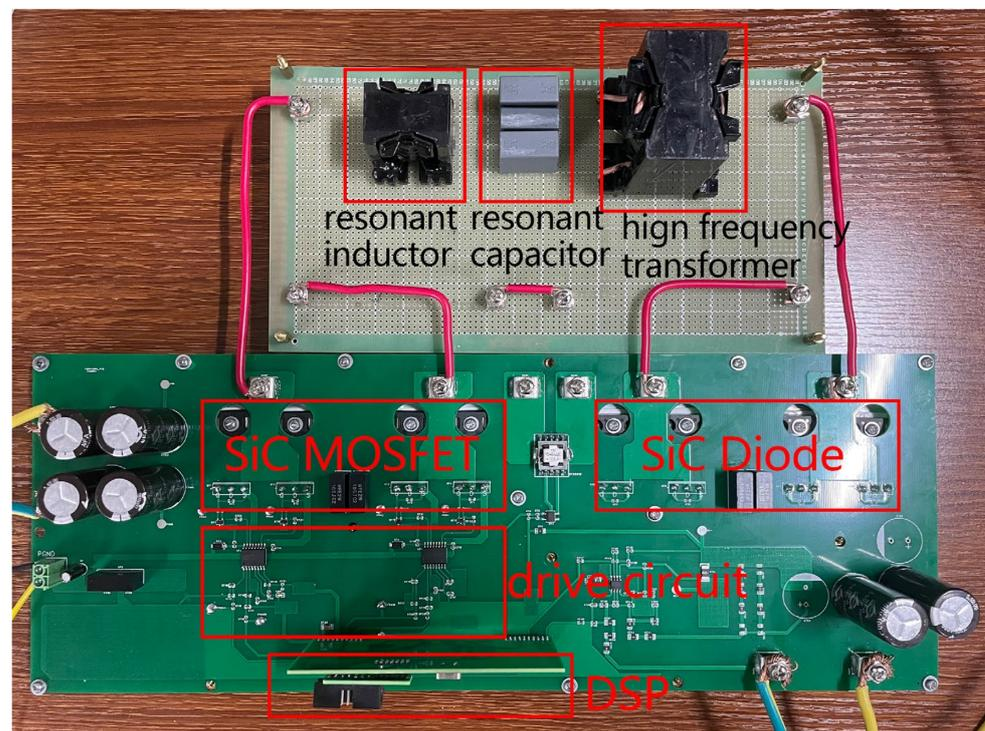
Figure 5. Experimental prototype.
