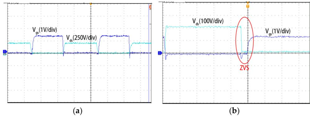
**Figure 10.** Experimental results for  $f_s = 125$  kHz: (a) Steady-state waveforms (time scale:  $2 \mu\text{s}/\text{div}$ ); (b) Soft-switching waveforms (time scale:  $800 \text{ ns}/\text{div}$ ).
