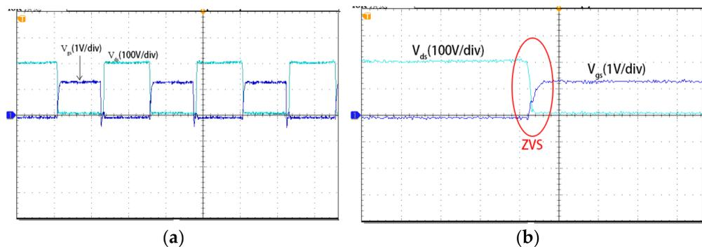
**Figure 9.** Experimental results for  $f_s = 100$  kHz: (a) Steady-state waveforms (time scale:  $4 \mu\text{s}/\text{div}$ ); (b) Soft-switching waveforms (time scale:  $800 \text{ ns}/\text{div}$ ).
