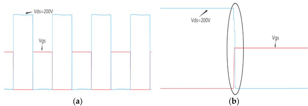
**Figure 6.** Simulation results for  $f_s = 100$  kHz: (a) Steady-state waveforms (time scale: 4  $\mu$ s/div); (b) partial amplification waveforms (time scale: 800 ns/div).
