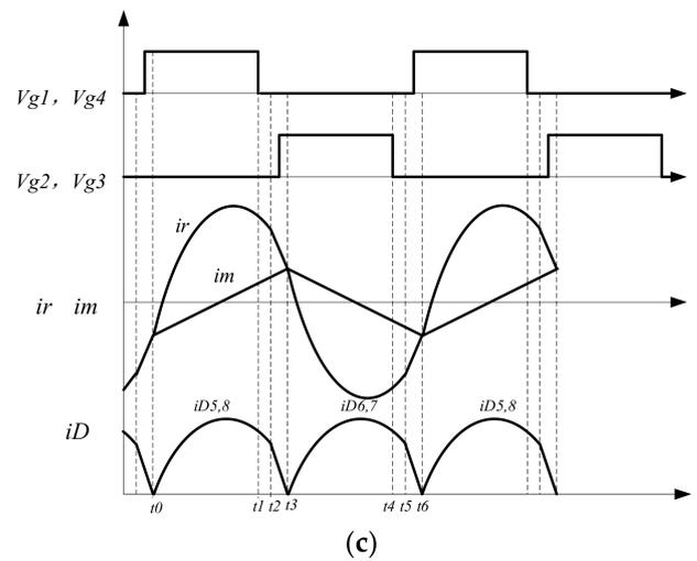
**Figure 2.** The working waveform of the full-bridge LLC resonant converter. (a)  $f_m < f_s < f_r$  (b)  $f_s = f_r$  (c)  $f_s > f_r$ .
