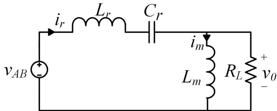
Figure 3. Equivalent circuit of the full-bridge LLC resonant converter.
