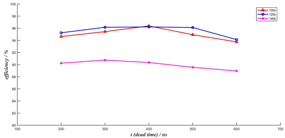
**Figure 12.** The relation curve between dead-time and efficiency.
