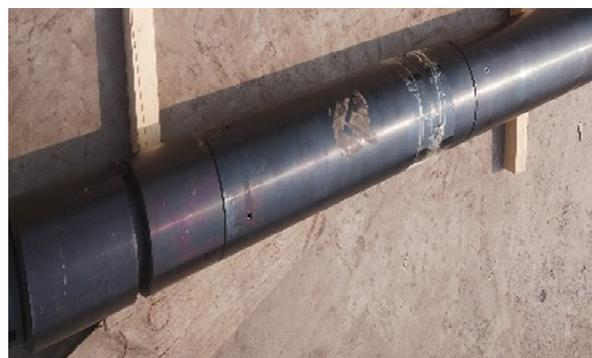
**Figure 9.** The prototype of the multi–source impact oscillation speed–increasing tool.
