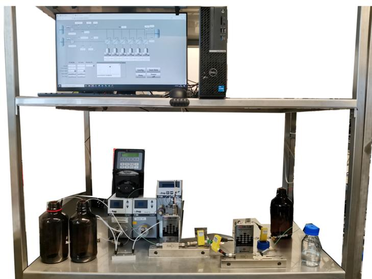
**Figure 26.** Set-up of the mixing section for the LNP formulation.
