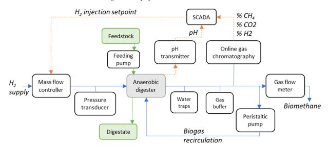
Figure 1. Schematic of the in-situ biomethanation experimental rig.
