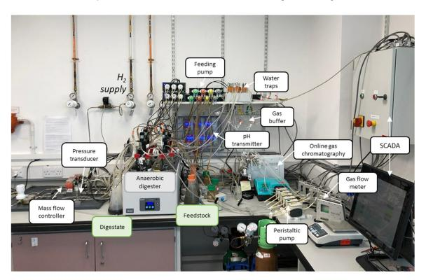
Figure 2. Photo of the in-situ biomethanation experimental rig with main components labelled.
