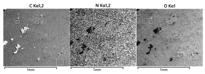
**Figure 4.** EDS image of CS-MB hydrogel. Conditions: Samples immobilized to carbon tape and coated with 5 nm of iridium for conductivity and then imaged at 5 kV.
