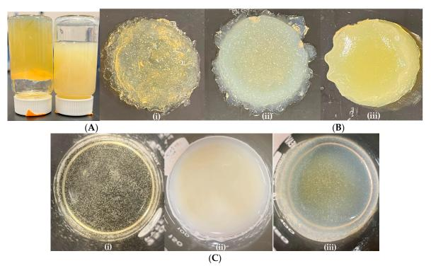
**Figure 1.** (**A**) Turbidity and viscosity of hydrogel solution at varying final CS concentrations post fabrication: (L) 2.1% w/v, (R) 1.7% w/v. (**B**) Hydrogel products after 16 h at varying component ratios: (i) 1 CS: 20 Glu: 20 4-HC, (ii) 1 CS: 30 Glu: 60 4-HC, (iii) 1 CS: 60 Glu: 120 4-HC. (**C**) Visual indications of successful CS-MB hydrogelation: (i) Pure CS gel in AcOH<sub>(aq)</sub>, (ii) incomplete/unsuccessful, (iii) complete/successful.
