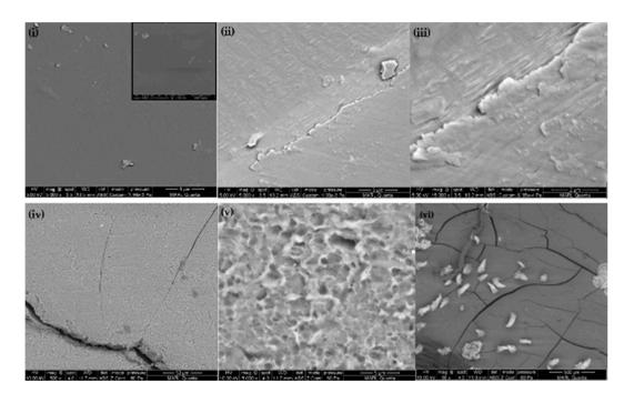
**Figure 3.** SEM images of CS-MB hydrogels: (i) CS film at  $5000 \times$ ; (ii) CS-MB at  $5000 \times$ ; (iii) CS-MB at  $15,000 \times$ ; (iv) CS-MB swollen in 5% w/v NaCl  $500 \times$ ; (v) CS-MB swollen in 5% w/v NaCl at  $5000 \times$ ; (vi) CS-MB swollen in 5% w/v NaCl at  $60 \times$  with visible NaCl on the surface.
