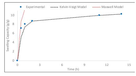
**Figure 5.** Fitting of experimental swelling capacity data with known model for viscoelastic polymeric materials. Conditions: 6.2 mg and thickness of 0.05 mm of hydrogel, 5 mL buffered solution at pH 4.0, and T = 22 °C.
