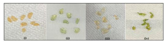
**Figure 9.** Fresh and Cu<sup>2+</sup> uptake spent hydrogels in their dry and swollen states: (i) fresh dry CS-MB; (ii) Cu<sup>2+</sup> uptake spent swollen CS-MB; (iii) fresh swollen CS-MB; (iv) Cu<sup>2+</sup> uptake spent dry CS-MB.
