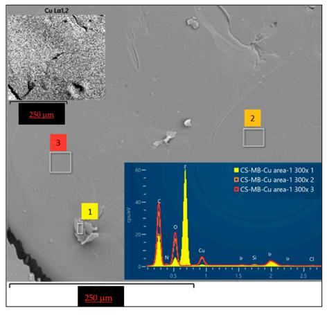
$Cu^{2+}$  on the surface of CS-MB means that there is no localization or aggregation of  $Cu^{2+}$ , but it adsorbed rather evenly at the surface, which is feasible for this application.
