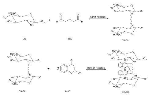
**Scheme 2.** Simplified mechanism of Mannich reaction (CS is represented as its glucosamine monomer).
