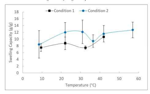
**Figure 7.** Effects of water temperature in the swelling capacity of CS-MB. Condition 1:  $6.0 \pm 2.0$  mg CS-MB immersion in 5 mL unbuffered distilled water for 0.5 h. Condition 2:  $4.5 \pm 1.5$  mg CS-MB, immersion in 5 mL pH 4 buffered solution for 11 h. The error bars represent standard deviation.
