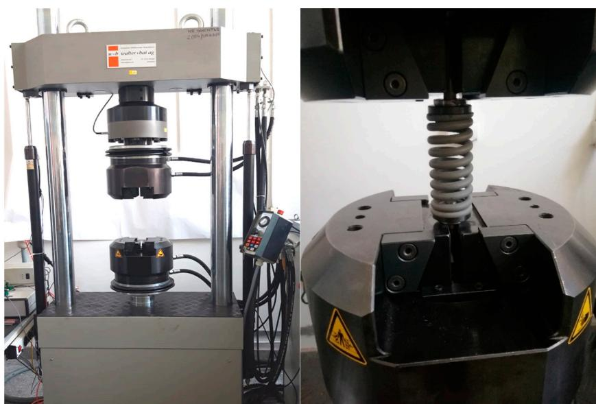
**Figure 4.** Determination of the elastic constant of the valve spring.
