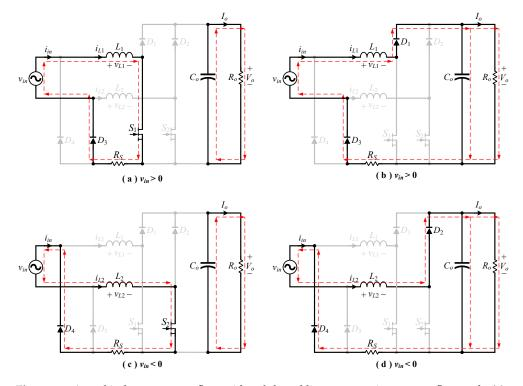
**Figure 13.** Actual inductor current flow with red dotted line representing current flow path: (a)  $v_{in} > 0$  and  $S_1$  on; (b)  $v_{in} > 0$  and  $S_1$  off; (c)  $v_{in} < 0$  and  $S_2$  on; (d)  $v_{in} < 0$  and  $S_2$  off.
