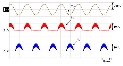
**Figure 16.** Inductor current under an input voltage of AC 115 V: (1)  $v_{in}$ ; (2)  $i_{L1}$ ; (3)  $i_{L2}$ .
