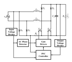
Figure 14. Overall system configuration.
