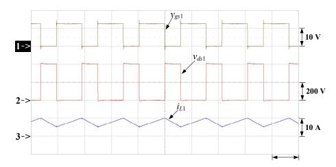
**Figure 24.** Measured waveforms at the input voltage AC 115 V peak: (1)  $v_{gs1}$ ; (2)  $v_{ds1}$ ; (3)  $i_{L1}$ .
