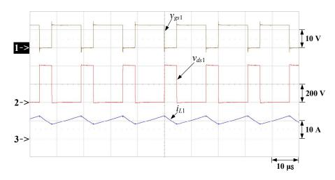
Figure 23. Measured waveforms at the input voltage AC 90 V peak: (1)  $v_{gs1}$ ; (2)  $v_{ds1}$ ; (3)  $i_{L1}$ .
