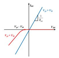
Figure 12. Operational characteristics of the GaNFET [31].
