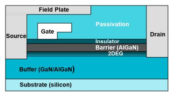
Figure 11. Cross-section of the GaNFET [31].
