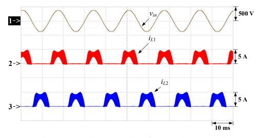
**Figure 18.** Inductor current under an input voltage of AC 264 V: (1)  $v_{in}$ ; (2)  $i_{L1}$ ; (3)  $i_{L2}$ .
