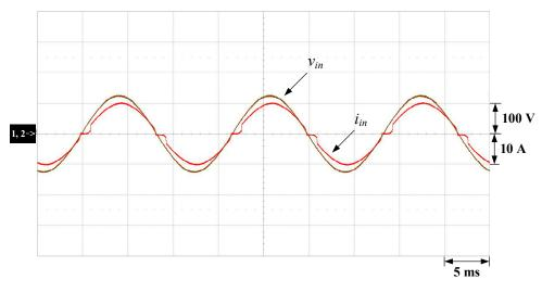
**Figure 19.** Input voltage and current under an input voltage of AC 90 V: (1)  $v_{in}$ ; (2)  $i_{in}$ .
