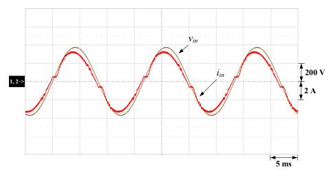
Figure 22. Input voltage and current under an input voltage of AC 264 V: (1)  $v_{in}$ ; (2)  $i_{in}$ .
