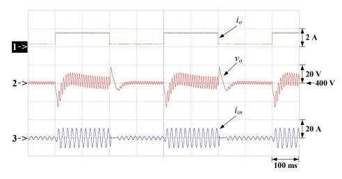
Figure 27. Dynamic response at an input voltage of AC 90 V: (1)  $i_0$ ; (2)  $v_0$ ; (3)  $i_{in}$ .
