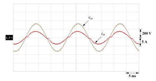
**Figure 21.** Input voltage and current under an input voltage of AC 230 V: (1)  $v_{in}$ ; (2)  $i_{in}$ .
