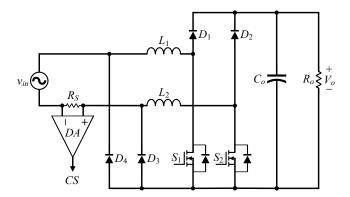
Figure 4. Inductor current detected by a differential amplifier.
