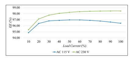
Figure 33. Curves of Eff. vs. load current under input voltages of 115 and 230 V.
