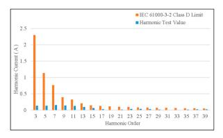
**Figure 34.** Comparison of current harmonic limit values and test values under an input voltage of AC 115 V.
