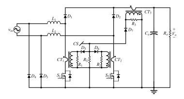
Figure 5. Inductor current detected by three transformers.
