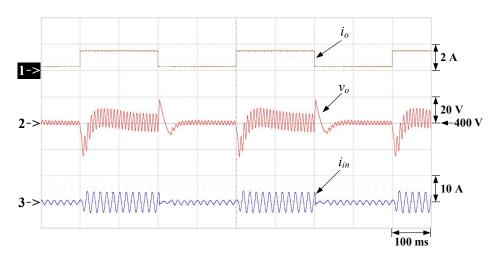
**Figure 29.** Dynamic response at an input voltage of AC 230 V: (1) *i*<sub>0</sub>; (2) *v*<sub>0</sub>; (3) *i*<sub>in</sub>.
