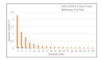
**Figure 35.** Comparison of current harmonic limit values and test values under an input voltage of AC 230 V.
