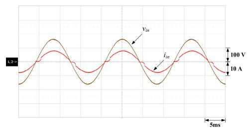
**Figure 20.** Input voltage and current under an input voltage of AC 115 V: (1)  $v_{in}$ ; (2)  $i_{in}$ .
