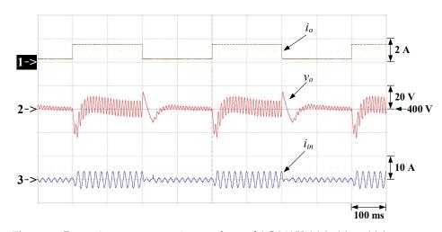
**Figure 30.** Dynamic response at an input voltage of AC 264 V: (1) *i*<sub>0</sub>; (2) *v*<sub>0</sub>; (3) *i*<sub>in</sub>.
