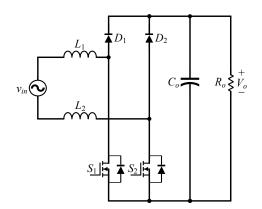
Figure 1. Basic, widely used semi-bridgeless PFC rectifier.
