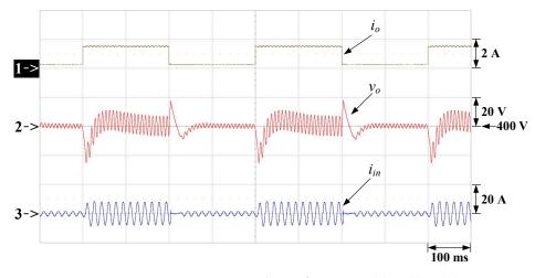
**Figure 28.** Dynamic response at an input voltage of AC 115 V: (1)  $i_0$ ; (2)  $v_0$ ; (3)  $i_{in}$ .
