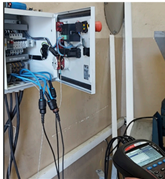
Figure 4. Portable electrical energy quality analyzer connected to the L1, L2, L3 current loops.
