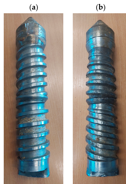
Figure 2. Extruder screw: (a) new (N), (b) worn-out (W).
