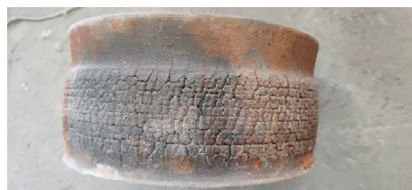
Figure 2. Roller wheel after high temperature failure (SUS304).
