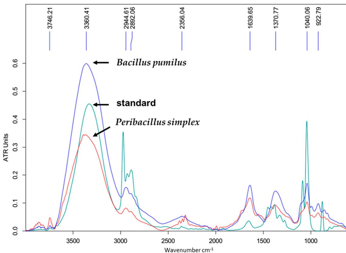
**Figure 4.** FTIR absorption spectra of biosurfactants, isolated from cultural medium of *B. pumilus* and *P. simplex* strain and of standard surfactin.
