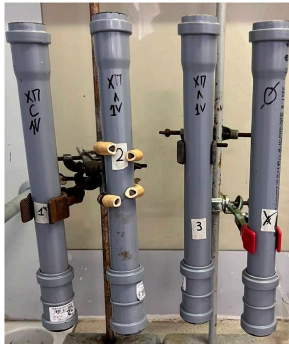
**Figure 1.** Sand-packed columns used to estimate the efficiency of biosurfactants for MEOR.
