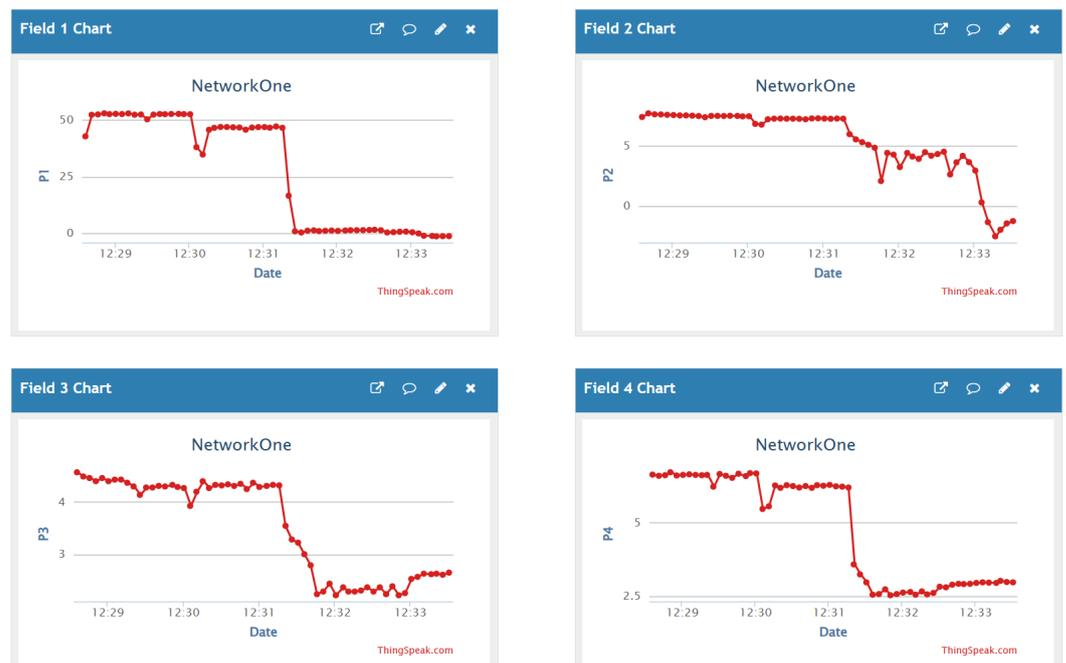
**Figure 7.** Real-time monitoring of the pressure head in the cloud environment (Fields 1 to 4 of the pressure head cloud channel).
