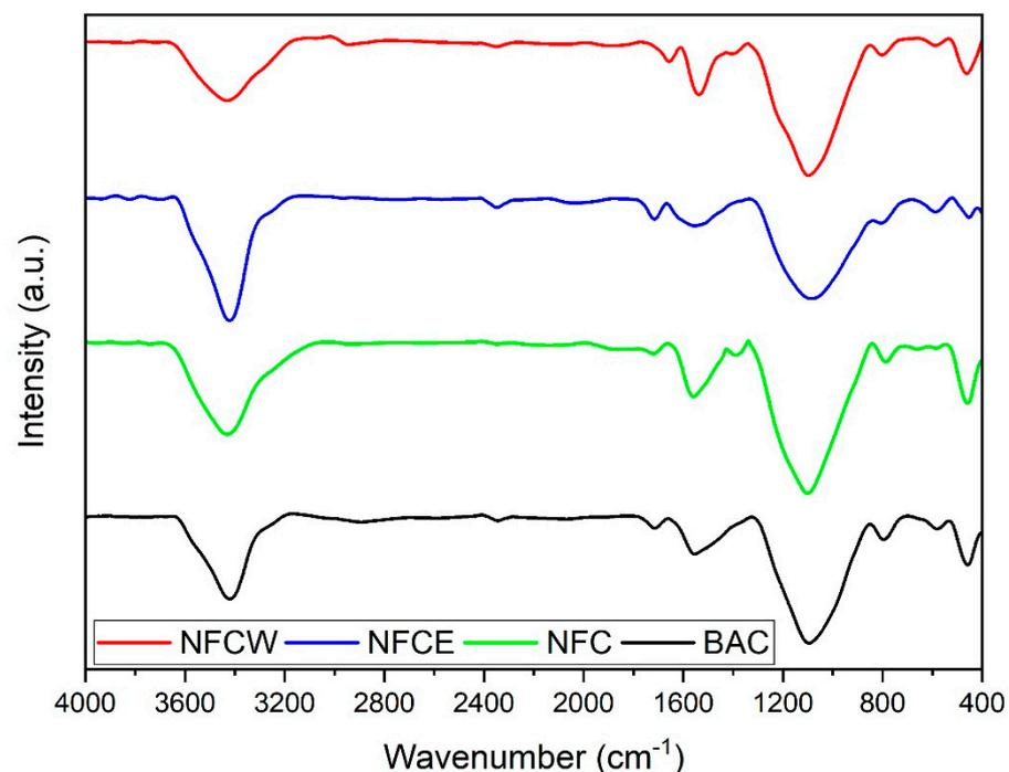
**Figure 2.** FTIR spectra of the activated carbon samples: NFCW (Nitric Functionalized Carbon impregnated with Water extract), NFCE (Nitric Functionalized Carbon impregnated with Ethanol extract), NFC (Nitric Functionalized Carbon), and BAC (Babassu Activated Carbon).
