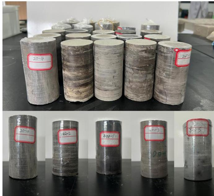
Figure 4. Appearance and morphology of mudstone after high temperature.
