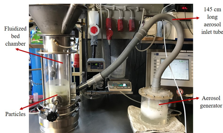
Figure 2. Experimental setup with 145 cm long aerosol inlet tube from the side of the fluidized bed.
