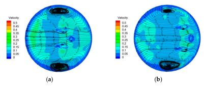
**Figure 10.** Streamline and velocity distribution of N1 section before and after optimization. (**a**) Before optimization. (**b**) After optimization.
