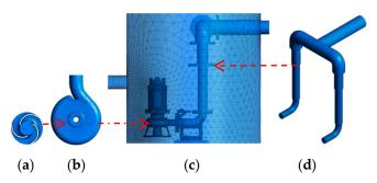
**Figure 2.** Grid diagram for each calculation area: (**a**) Impeller; (**b**) Volute Casing; (**c**) Centrifugal prefabricated pumping station; (**d**) Outlet section.
