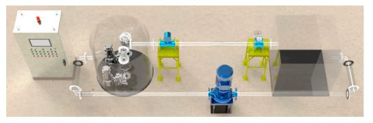
Figure 4. Centrifugal prefabricated pumping station 3D model diagram.
