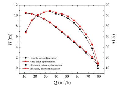
Figure 8. Comparison of energy characteristics before and after optimization.
