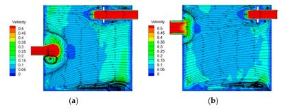
**Figure 12.** Streamline and velocity distribution of N3 section before and after optimization. (**a**) Before optimization. (**b**) After optimization.
