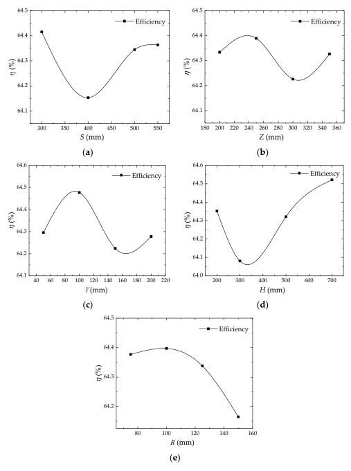
**Figure 7.** Prefabricated pumping station efficiency and each factor of the relationship curve. (**a**) Pump spacing *S*. (**b**) Suspended height *Z*. (**c**) Center spacing *Y*. (**d**) Inlet height *H*. (**e**) Inlet radius *R*.
