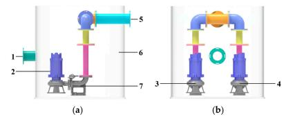
**Figure 1.** The 3D model structure of centrifugal prefabricated pumping station: 1. Inlet; 2. Motor; 3. Submersible centrifugal pump A; 4. Submersible centrifugal pump B; 5. Outlet; 6. Prefabricated barrel; 7. Coupler. (**a**) Side view. (**b**) Front view.
