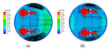
**Figure 11.** Streamline and velocity distribution of N2 section before and after optimization. (**a**) Before optimization. (**b**) After optimization.
