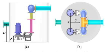
**Figure 6.** Schematic diagram of optimized parameters of prefabricated pumping station. (**a**) Side view. (**b**) Top view.
