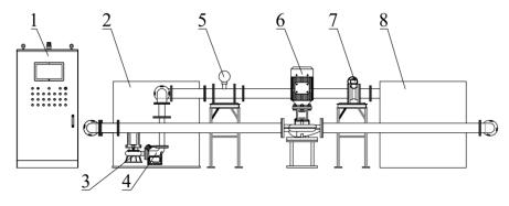
**Figure 3.** Sketch of centrifugal prefabricated pumping station test bench: 1. PLC frequency conversion control cabinet; 2. Prefabricated barrel; 3. Submersible centrifugal pump; 4. Coupler; 5. Electromagnetic flow meter; 6. Pipeline pump; 7. Butterfly valve; 8. Water return tank.
