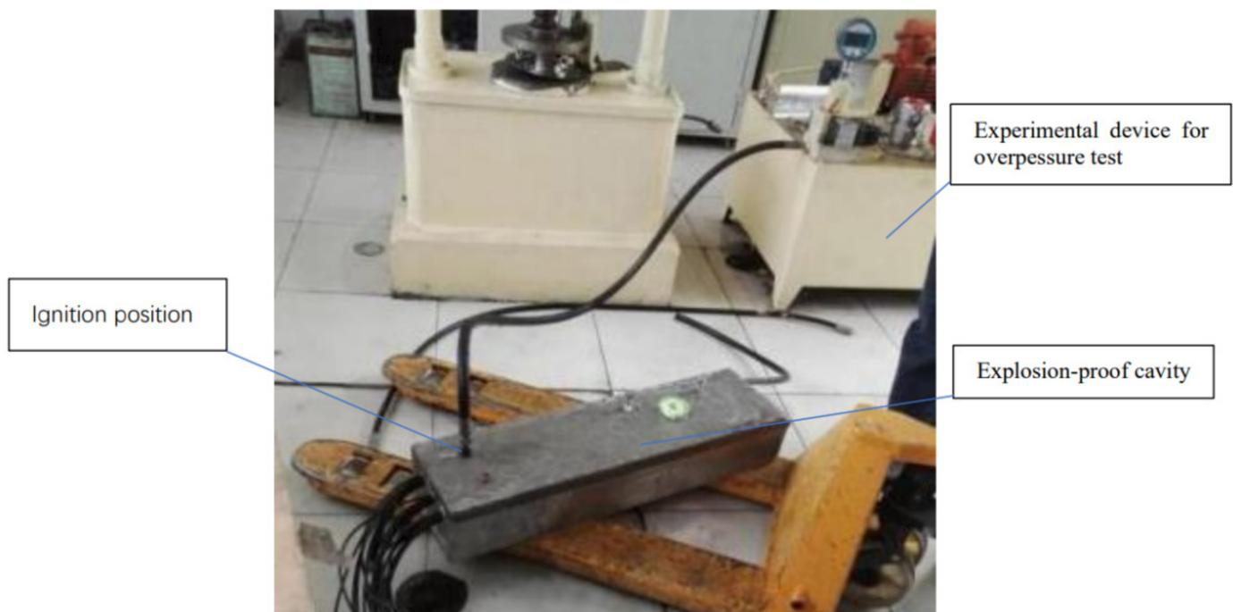
**Figure 20.** Testing setup of pressure test.
