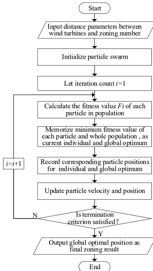
Figure 1. Improved DPSO algorithm.
