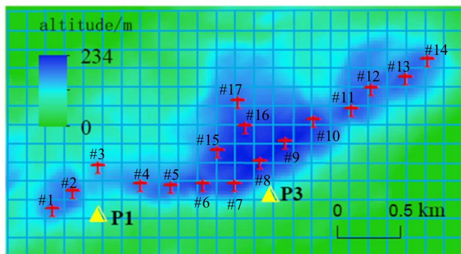
Figure 12. Optimal location of wind monitoring point.
