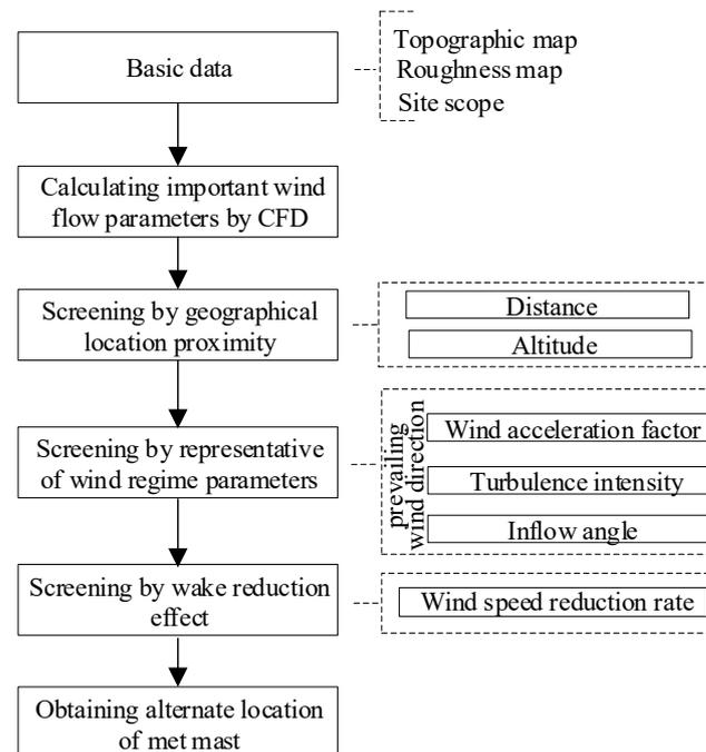
**Figure 2.** Location screening process of alternative met mast.
