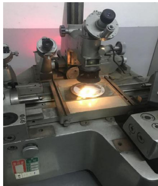
Figure 6. Universal tool microscope of the 19J(JX7) type.
