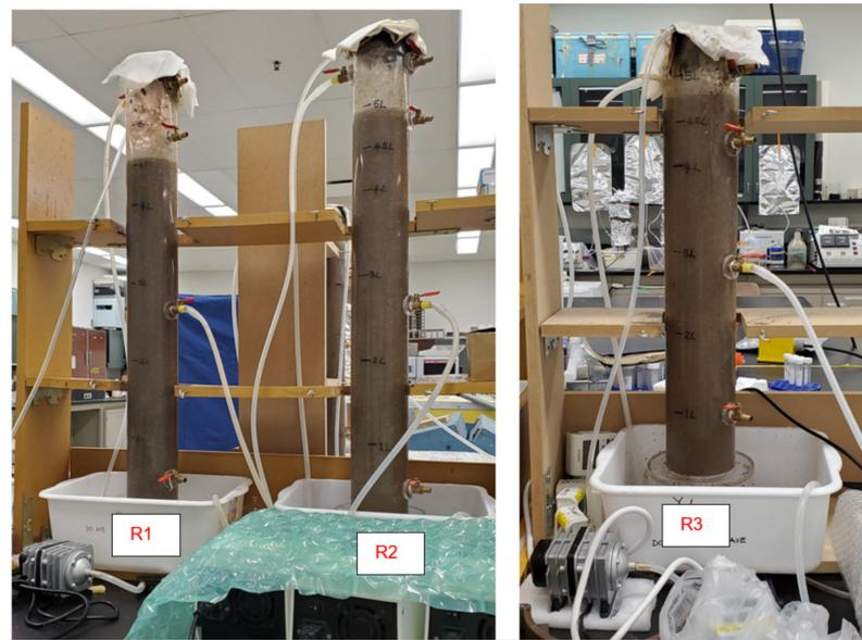
Figure 1. AGS bioreactors (R1, R2, R3) in operation.
