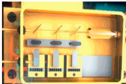
**Figure 2.** Optical coupled pump LD.
