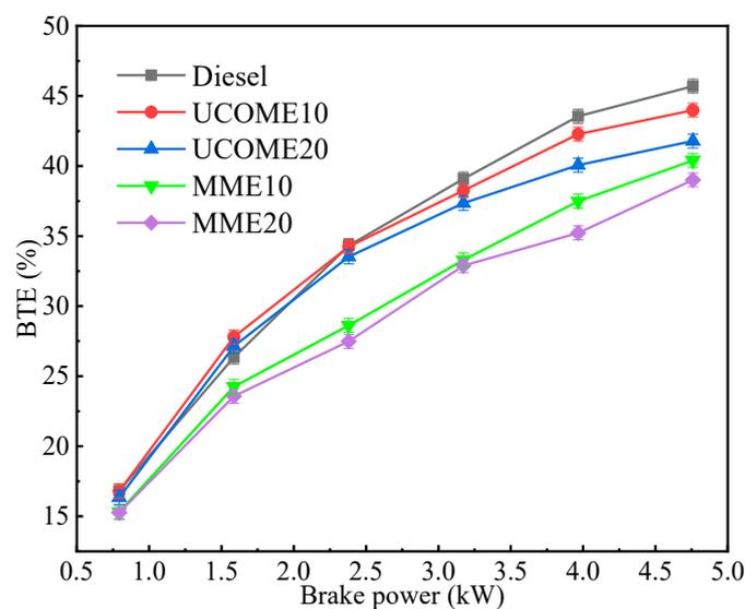
Figure 14. BTE comparison of mustard oil used cooking oil and diesel under different loads [173].
