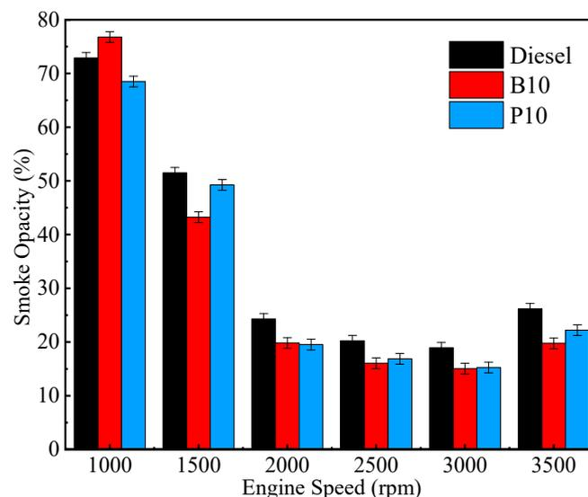
**Figure 34.** Smoke emission comparison of biodiesel blends and diesel at different engine speeds [258].
