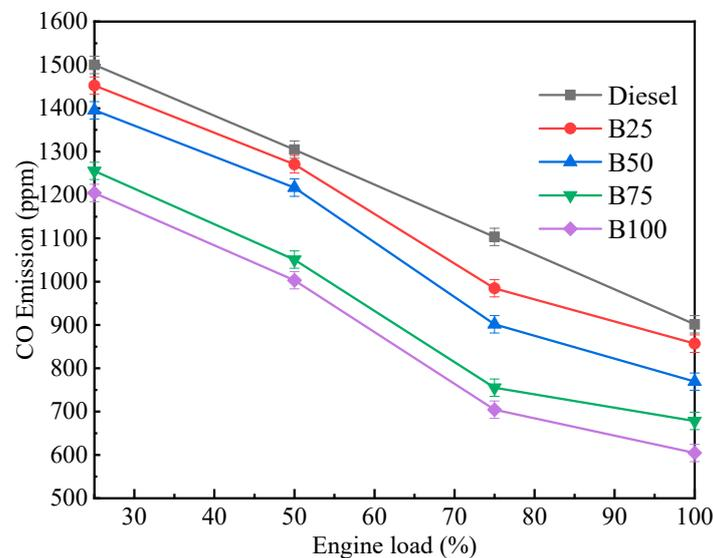
**Figure 23.** CO emission comparison of biodiesel blends and diesel under different engine loads [226].
