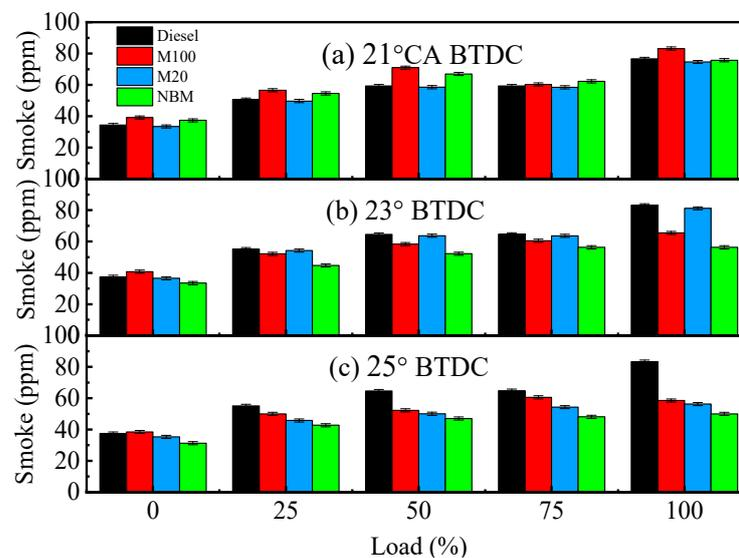
Figure 33. Smoke emission of NBM biodiesel blends and diesel under different loads [257].
