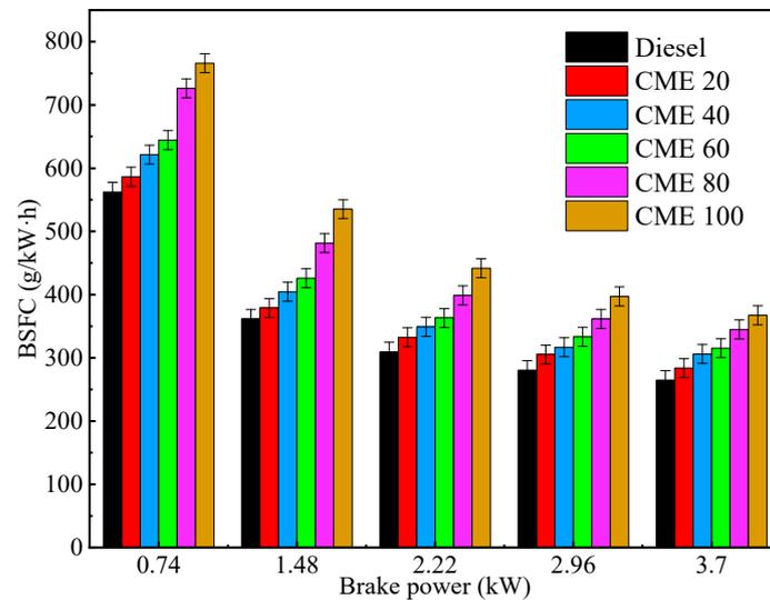
Figure 18. BSFC comparison of CME blends and diesel under different brake powers [185].
