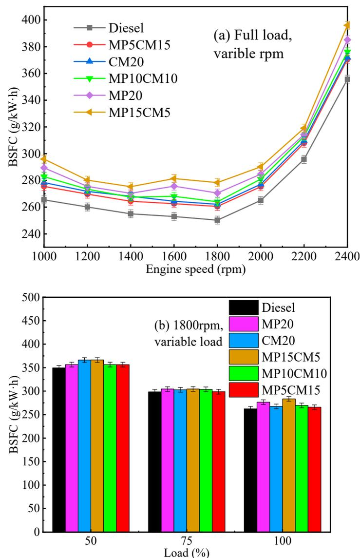
Figure 17. BSFC at different engine conditions. (a) Different speeds; (b) Different loads [193].
