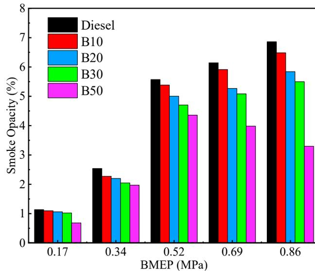
Figure 32. Smoke emission comparison of biodiesel blends and diesel under different BMEPs [169].
