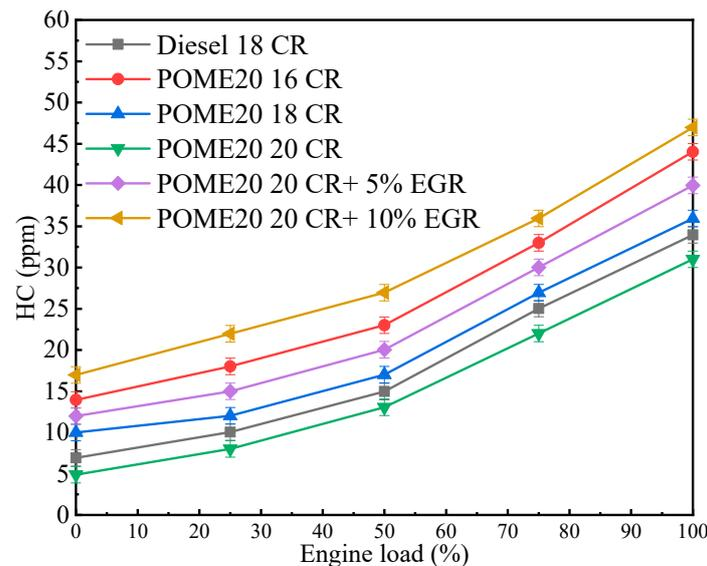
**Figure 31.** HC emission comparison of POME biodiesel and diesel under different loads [241].
