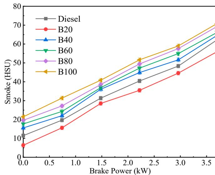
**Figure 35.** Smoke emission comparison of castor biodiesel blends and diesel under different brake powers [185].
