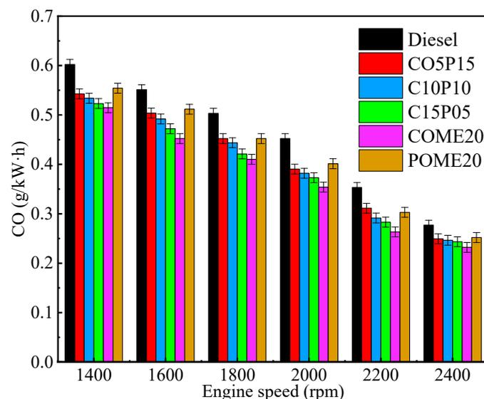
**Figure 21.** CO emission comparison of COME and POME biodiesel blends at different engine speeds [222].
