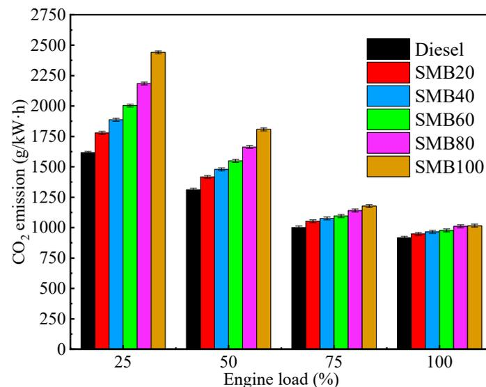
**Figure 24.** CO<sub>2</sub> emission comparison of SME biodiesel and diesel under different loads [231].
