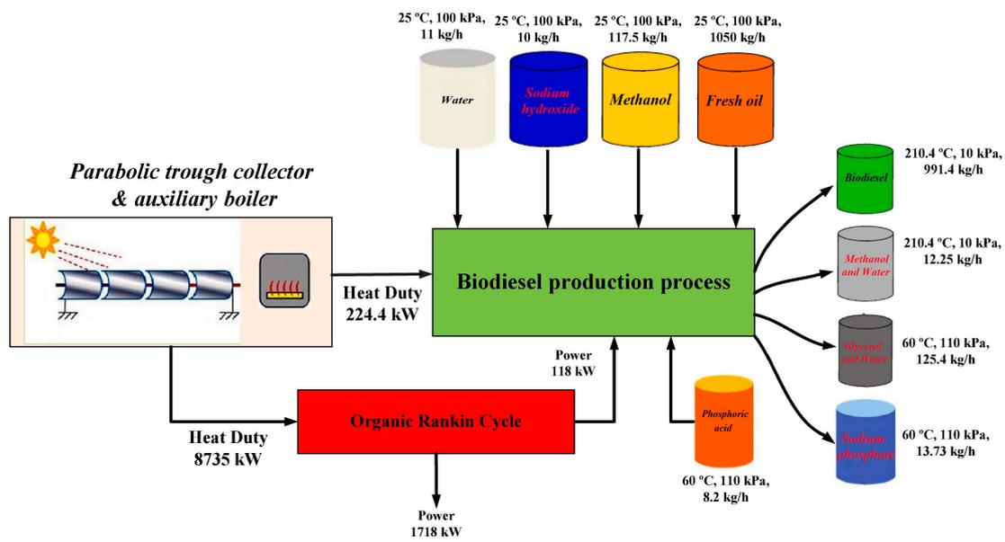
Figure 11. Biodiesel production using parabolic trough solar collectors [159].
