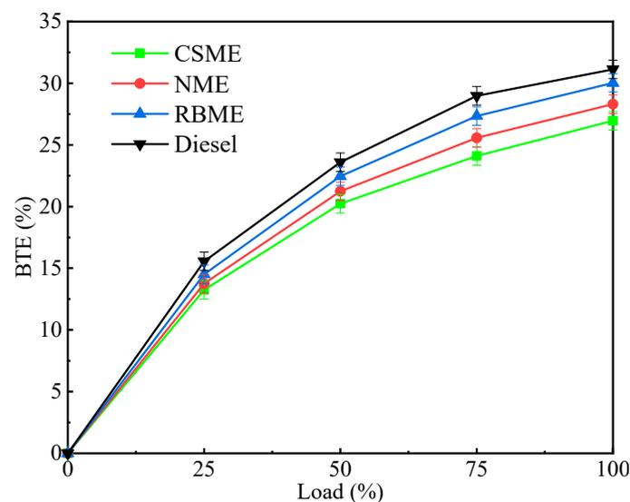
**Figure 15.** BTE comparison of three different biodiesels and diesel under different loads [183].
