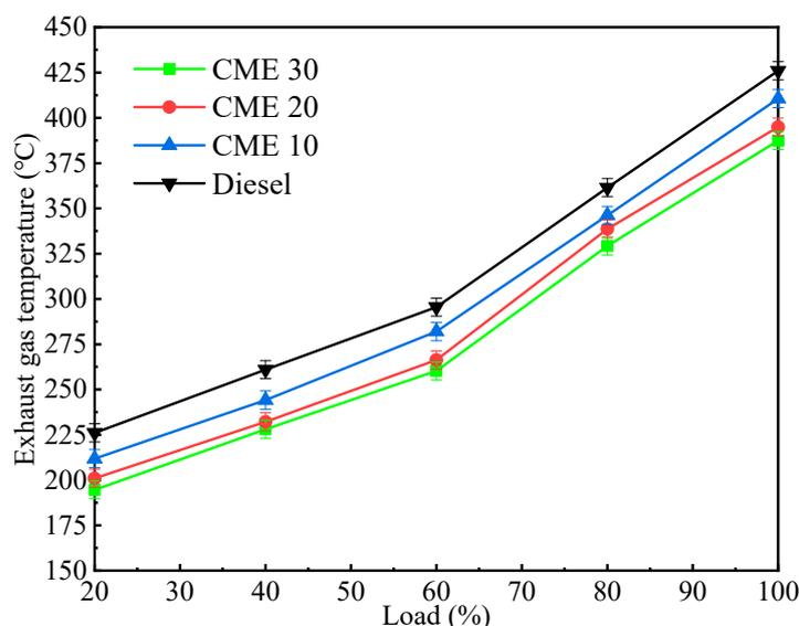
Figure 19. EGT comparison of CME biodiesel blends and diesel under different loads [210].
