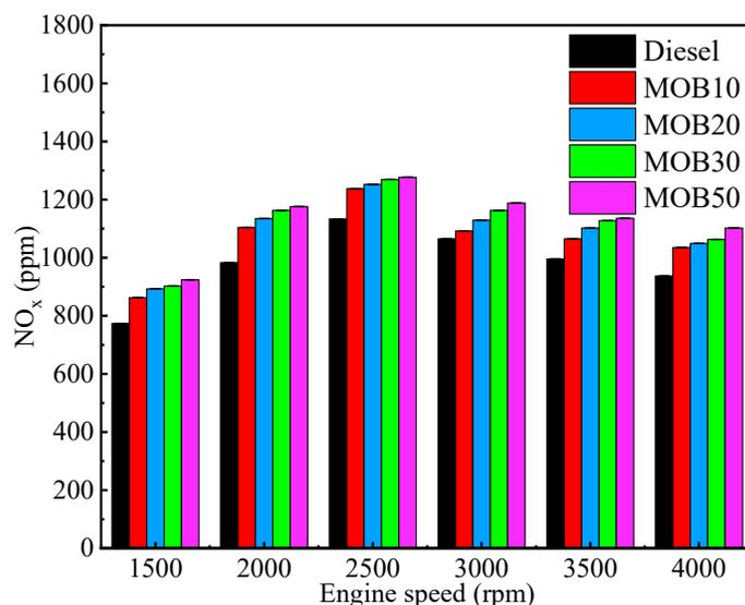
**Figure 28.**  $\text{NO}_x$  emissions comparison of MOB biodiesel blends and diesel at different engine speeds [172].
