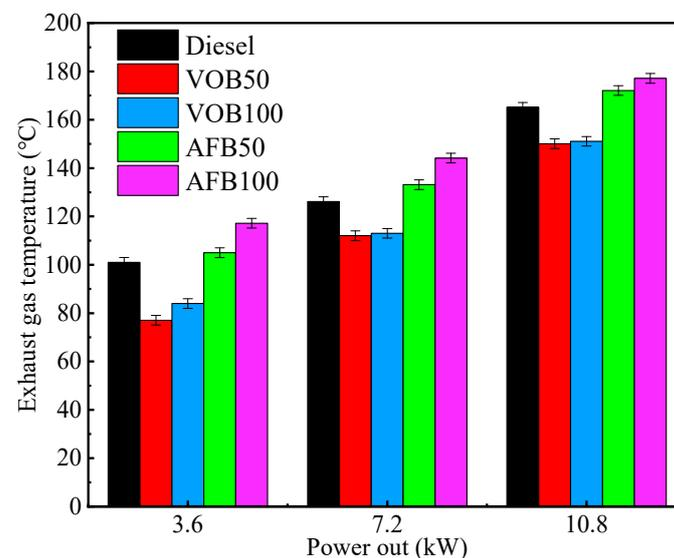
**Figure 20.** EGT comparison of AFB biodiesel and VOB biodiesel blends under different brake powers [214].
