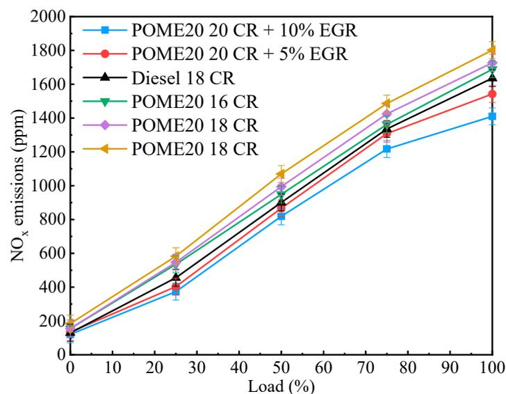
Figure 27.  $\text{NO}_x$  emissions comparison of POME biodiesel blends and diesel under different loads [241].
