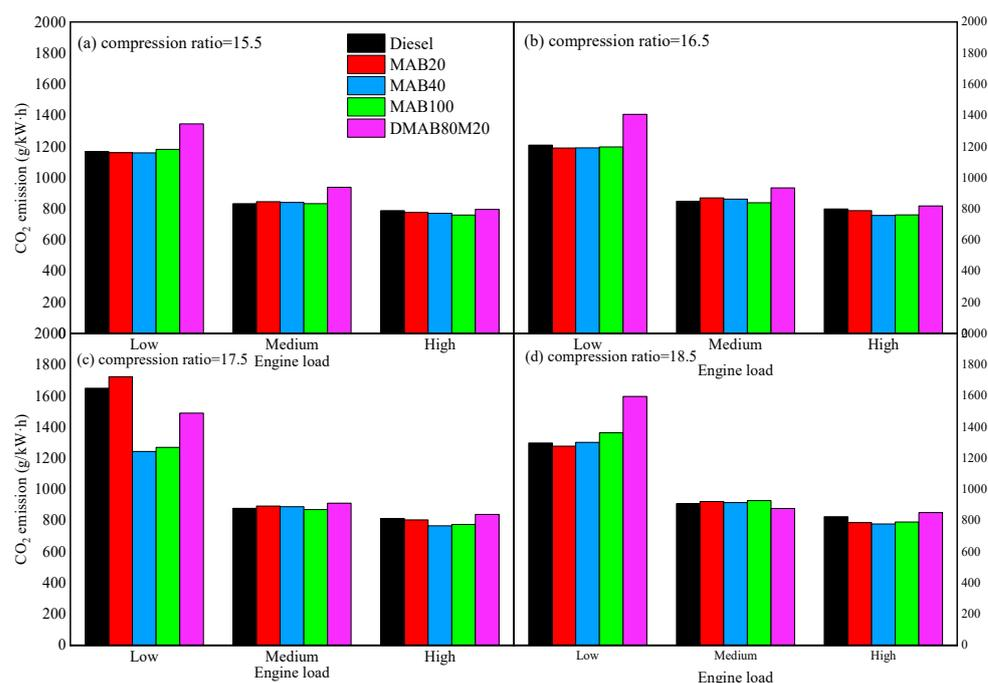
**Figure 26.** CO<sub>2</sub> emission comparison of biodiesel and diesel under different engine loads [231].
