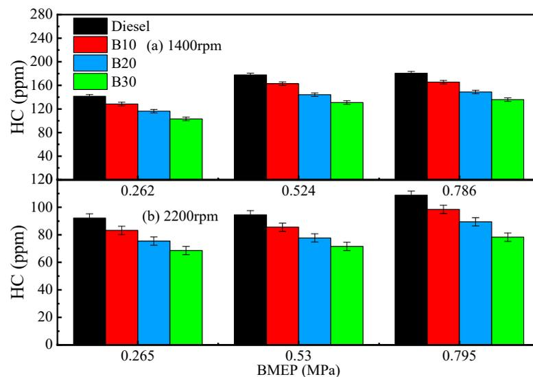
**Figure 29.** HC emission comparison of biodiesel blends and diesel under different BEMPs [180]. (a) 1400 rpm; (b) 2200 rpm.
