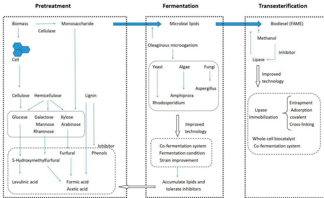
Figure 12. The Production process of using microorganisms to produce biodiesel [162].
