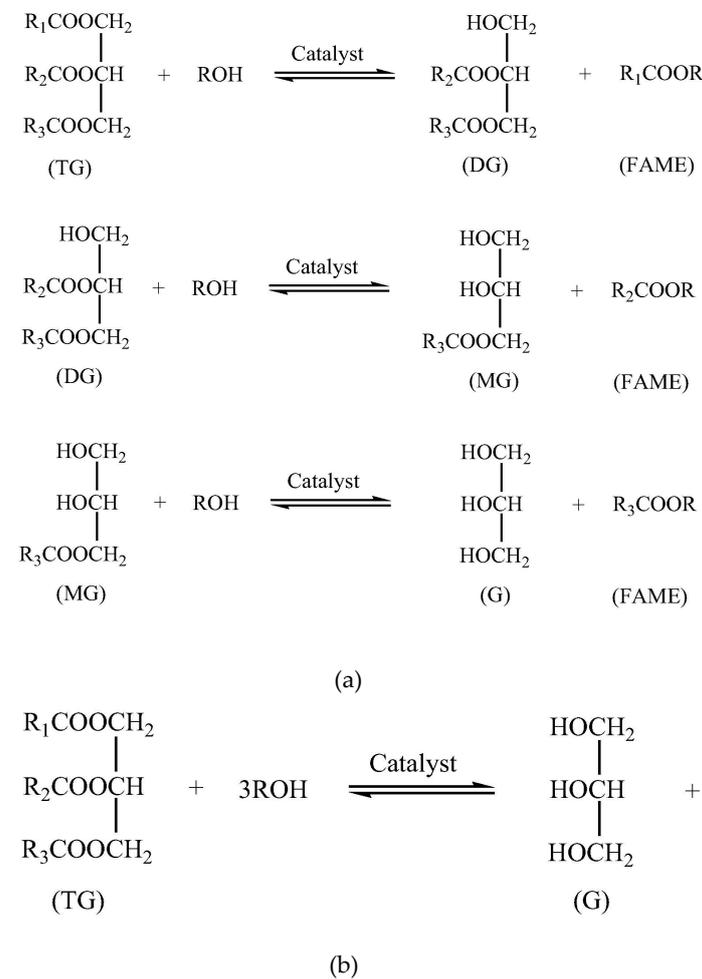
**Figure 4.** Transesterification reaction process [64]. (a) Transesterification of triglycerides; (b) Fast transesterification of triglycerides.
