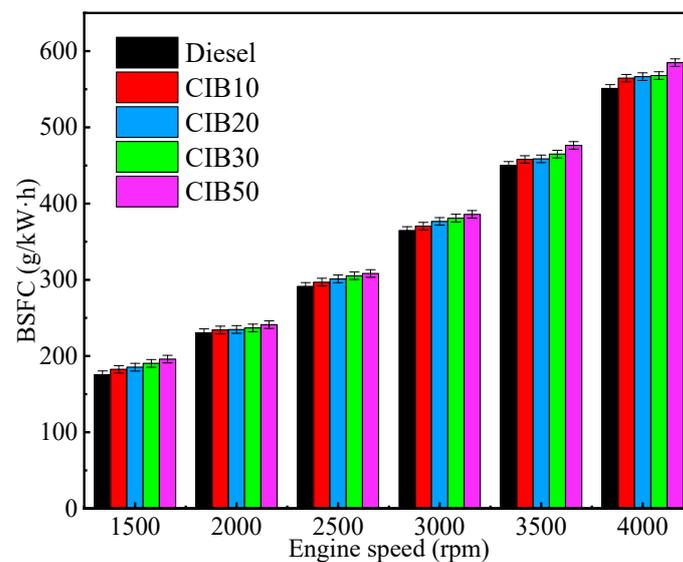
Figure 16. BSFC comparison of CIB biodiesel and diesel at different engine speeds [189].
