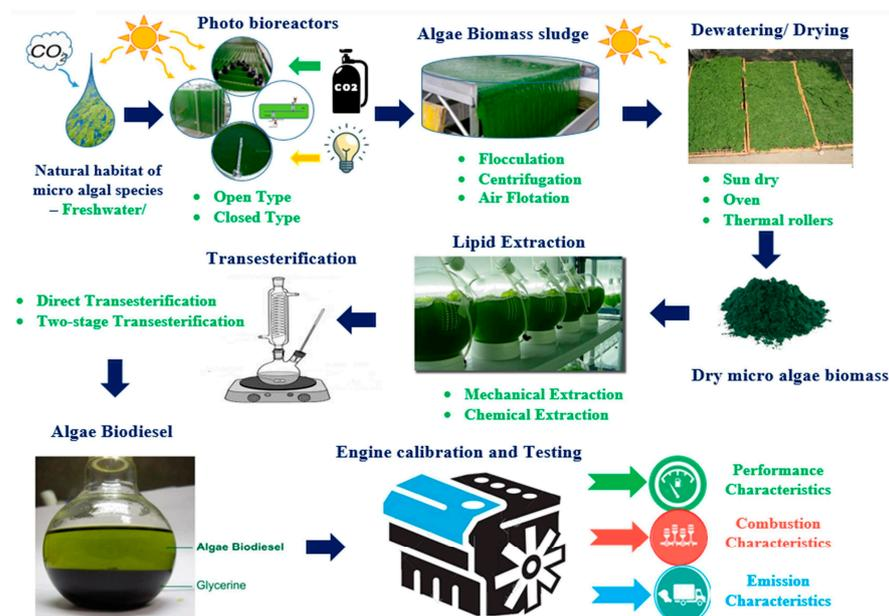
Figure 10. Micro-algal biodiesel production technique and components in processing [143].
