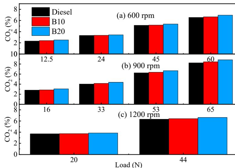
**Figure 25.** CO<sub>2</sub> emission comparison of biodiesel blends and diesel under different loads [197].
