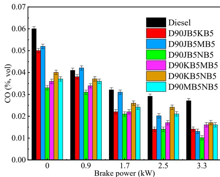
**Figure 22.** CO emission comparison of two biodiesel blends and diesel under different brake powers [217].
