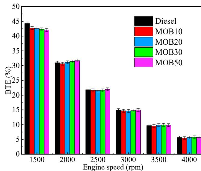
Figure 13. BTE of Moringa oil biodiesel blends at different engine speeds [172].
