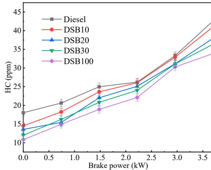
**Figure 30.** HC emission comparison of biodiesel blends and diesel under different brake powers [191].
