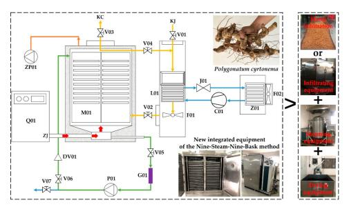
**Figure 1.** Working principle and basic composition of the new integrated equipment of the Nine-Steam-Nine-Bask method.
