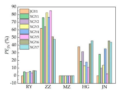
**Figure 13.** Total processing electric energy percentage of the product for infiltrating, steaming, braising, and drying under different processing conditions and the percentage of electric energy savings compared with JGY1.
