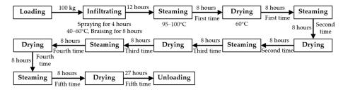
Figure 4. Processing flow of process 2 of the new equipment (New Process 2, XGY2).
