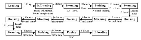
Figure 2. Processing flow of process 1 of the old equipment (Old Process 1, JGY1).
