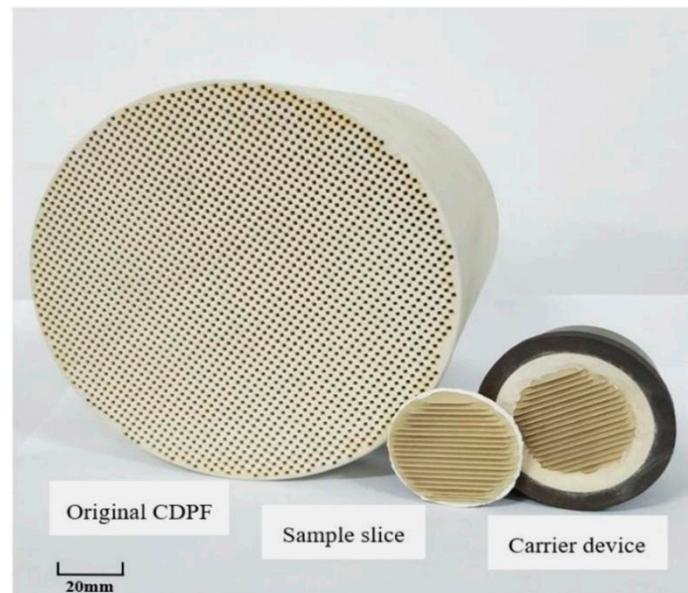
**Figure 7.** The original CDPF, sample slice, and carrier device [91].
