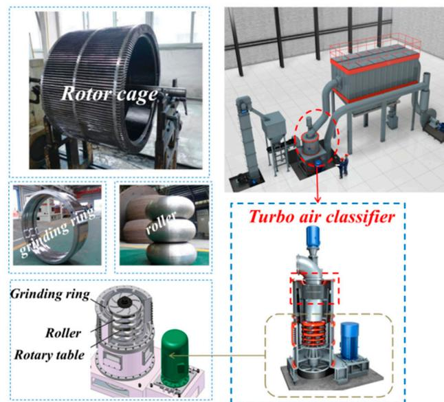
**Figure 2.** Scheme diagram of the pneumatic screening system.
