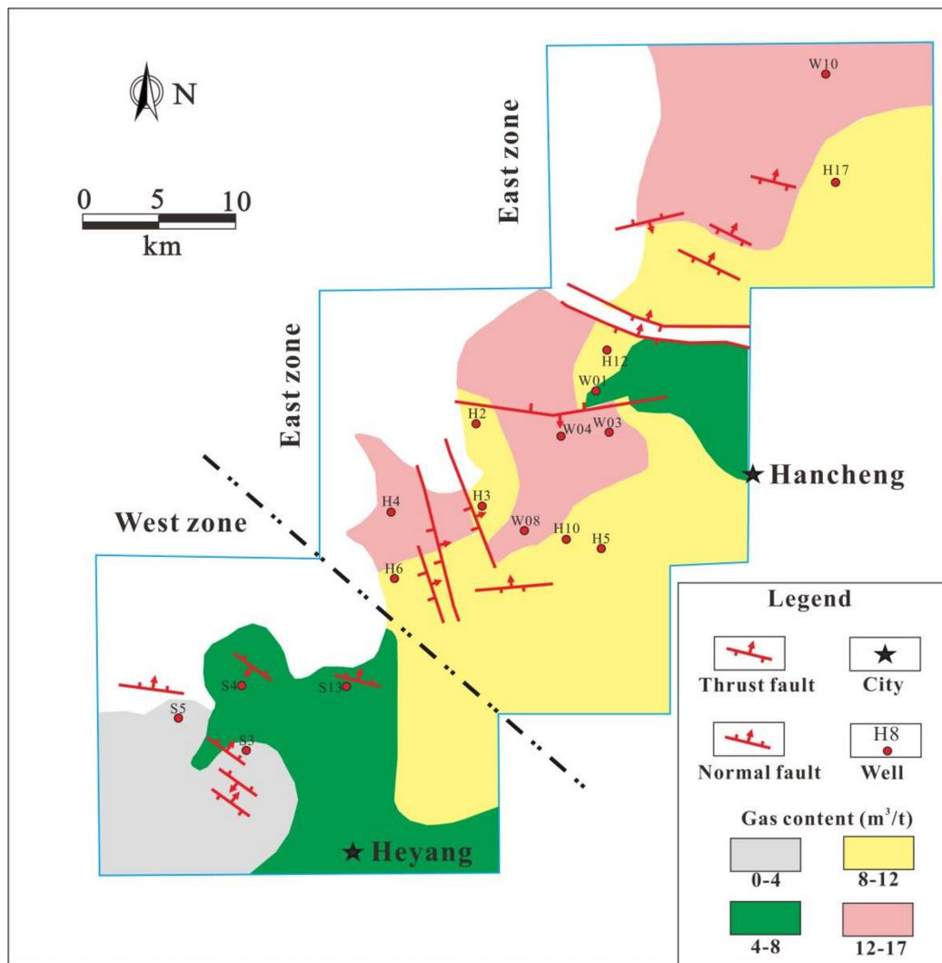
**Figure 4.** The distribution of gas content of the No.5 coal seam in the Weibei Field.
