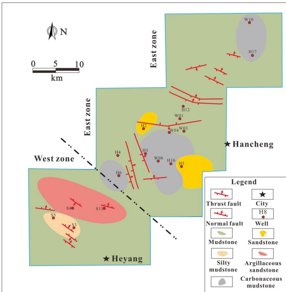
Figure 5. Roof lithology distribution of the No.5 coal seam in the Weiwei Field.
