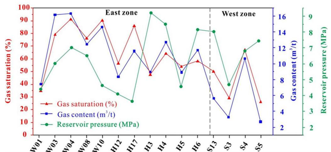
**Figure 11.** Relationship of gas content, gas saturation, and reservoir pressure of the No.5 coal seam in the Weibei Field.
