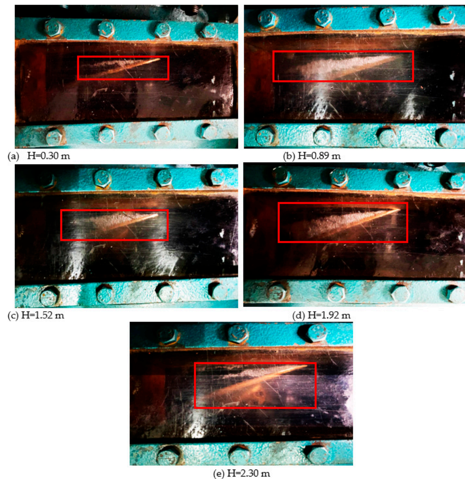
Figure 8. Cavitation diagram under five characteristic heads ( -4^\circ ).
