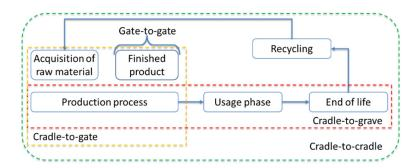
Figure 4. LCA boundary system approach.
