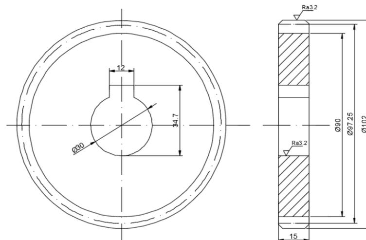
Figure 7. Gear dimension drawing.
