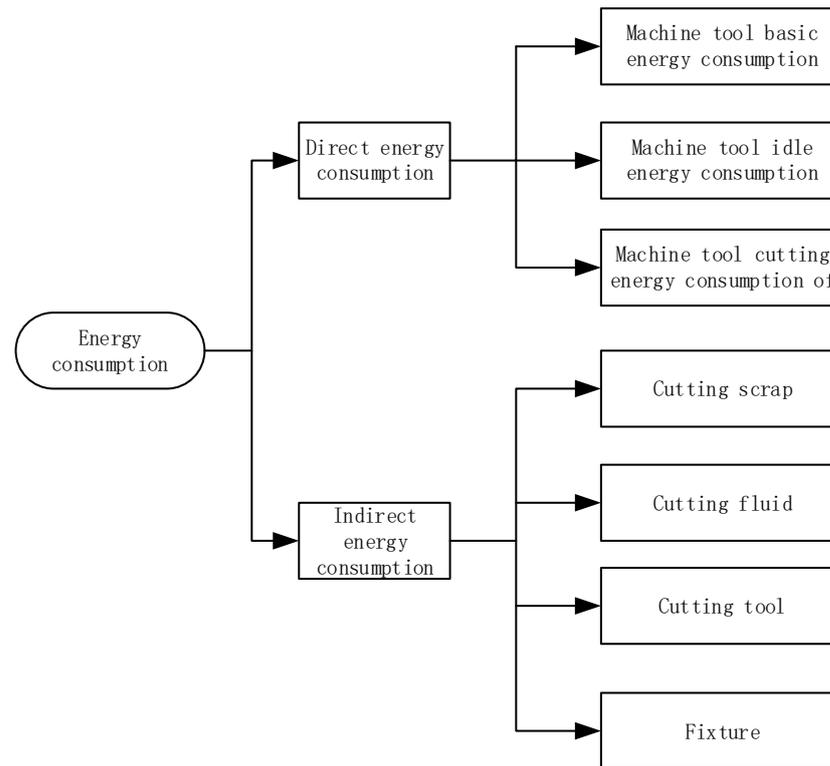
**Figure 1.** Influencing factors of energy consumption in gear machining process.
