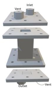
**Figure 2.** Different components of a  $z^2$  cuboid SEC device.
