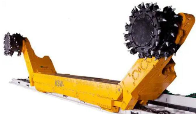
**Figure 1.** KSW-460NE shearer machine.
