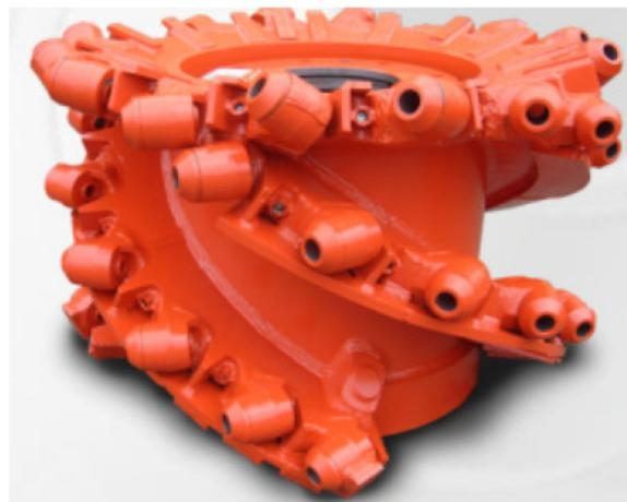
**Figure 2.** Cutter drum of the shearer machine.
