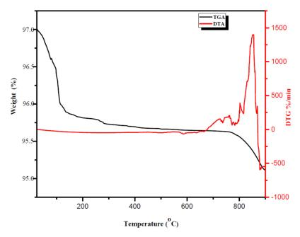
Figure 7. TGA-DTA curves of SNP<sub>s</sub>.
