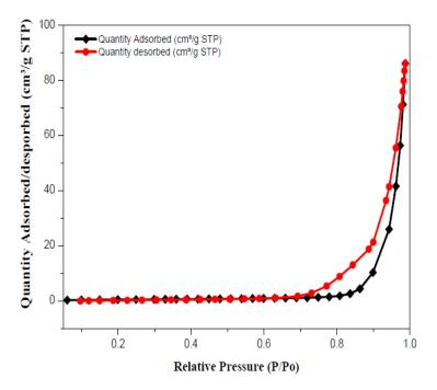
Figure 8. Adsorption–desorption SNPs isotherms of  $N_2$ .
