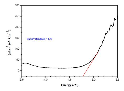
**Figure 6.** The energy band gap of extracted SNPs.
