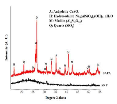
Figure 2. XRD analysis of SAFA and SNP.
