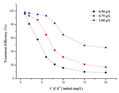
**Figure 11.** Original concentrations of  $Cd^{2+}$  as a function of SNPs removal efficiency (T = 30  $^{\circ}$ C, pH = 5).
