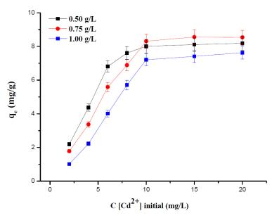
**Figure 10.** The initial concentrations of  $Cd^{2+}$  as a function of SNPs dosage (T = 30  $^{\circ}$ C, pH = 5).
