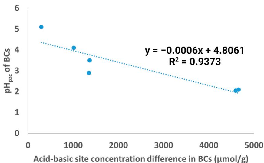
**Figure 5.** Correlation between the difference in acidic-basic site concentration and pH<sub>pzc</sub> of biochar samples.
