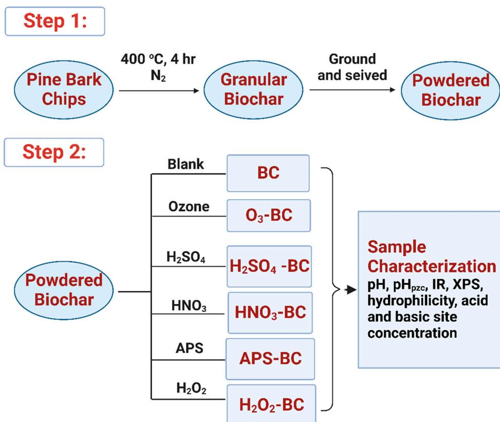
**Figure 1.** Schematic diagram showing the preparation and characterization techniques of biochar samples.
