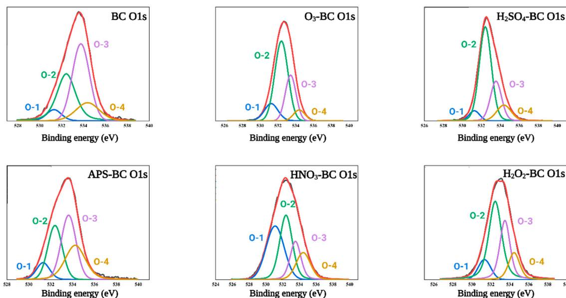
**Figure 4.** Deconvolution of O1s spectra for all the biochar samples. O-1: carbonyl and quinone; O-2: esters and anhydrides; O-3: ether-type oxygen in esters and anhydrides; and O-4: carboxylic oxygen.
