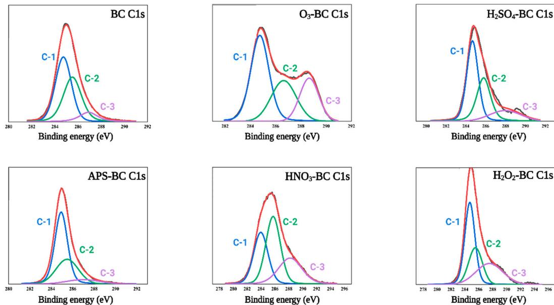
**Figure 3.** Deconvolution of C1s spectra for all the biochar samples. C-1:  $sp^2$  hybridized carbon; C-2: C-O bonds; C-3: C=O bonds.
