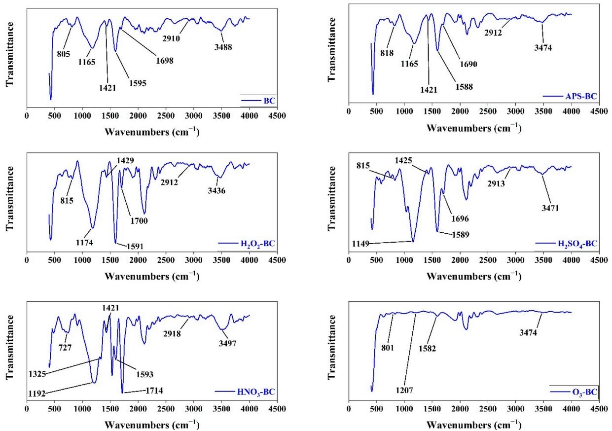
Figure 2. IR Spectra of BC, APS-BC, H<sub>2</sub>O<sub>2</sub>-BC, H<sub>2</sub>SO<sub>4</sub>-BC, HNO<sub>3</sub>-BC, O<sub>3</sub>-BC.
