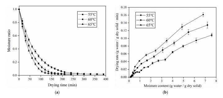
**Figure 2.** Moisture ratio (**a**) and drying rate (**b**) curves of cantaloupe slices under different SMIR drying temperatures (slice thickness 7 mm, radiation distance 120 mm).
