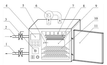
**Figure 1.** Schematic of the short- and medium-wave infra-red dryer. 1. wet discharging port, 2. air inlet port, 3. wind speed adjusting knob, 4. touch screen, 5. temperature sensor, 6. centrifugal fan, 7. spray nozzle 8. quartz infrared heating tube, 9. drying chamber, 10. material tray, 11. door.
