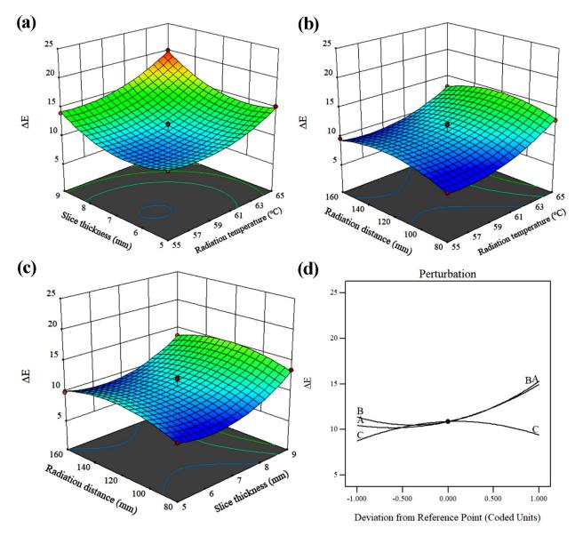
**Figure 5.** Response surface (**a**–**c**) and perturbation plot (**d**) for the effects of variables on the  $\Delta E$  of cantaloupe slices.
