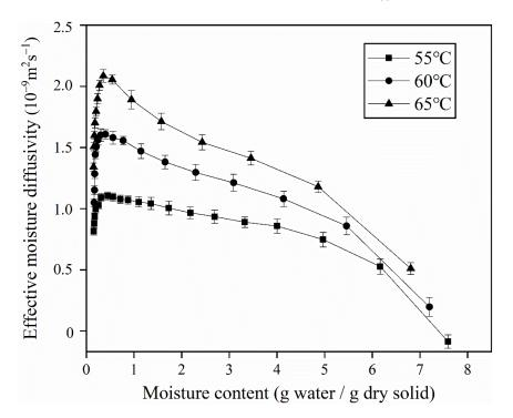
**Figure 3.** Effective moisture diffusivity versus moisture content of cantaloupe slices under different SMIR drying temperatures (slice thickness 7 mm, radiation distance 120 m).
