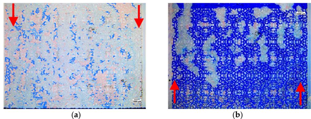
**Figure 9.** The subsequent water invasion process diagram after polymer microsphere injection and microsphere expansion in the homogeneous model. (a) The microsphere is injected along the simulated “horizontal wellbore”; (b) end of the second water flooding.
