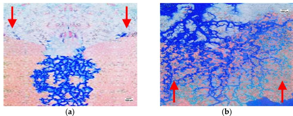
**Figure 13.** Process diagram of heterogeneous model gel injection and subsequent water flooding. (a) gel injection, (b) subsequent water flooding.
