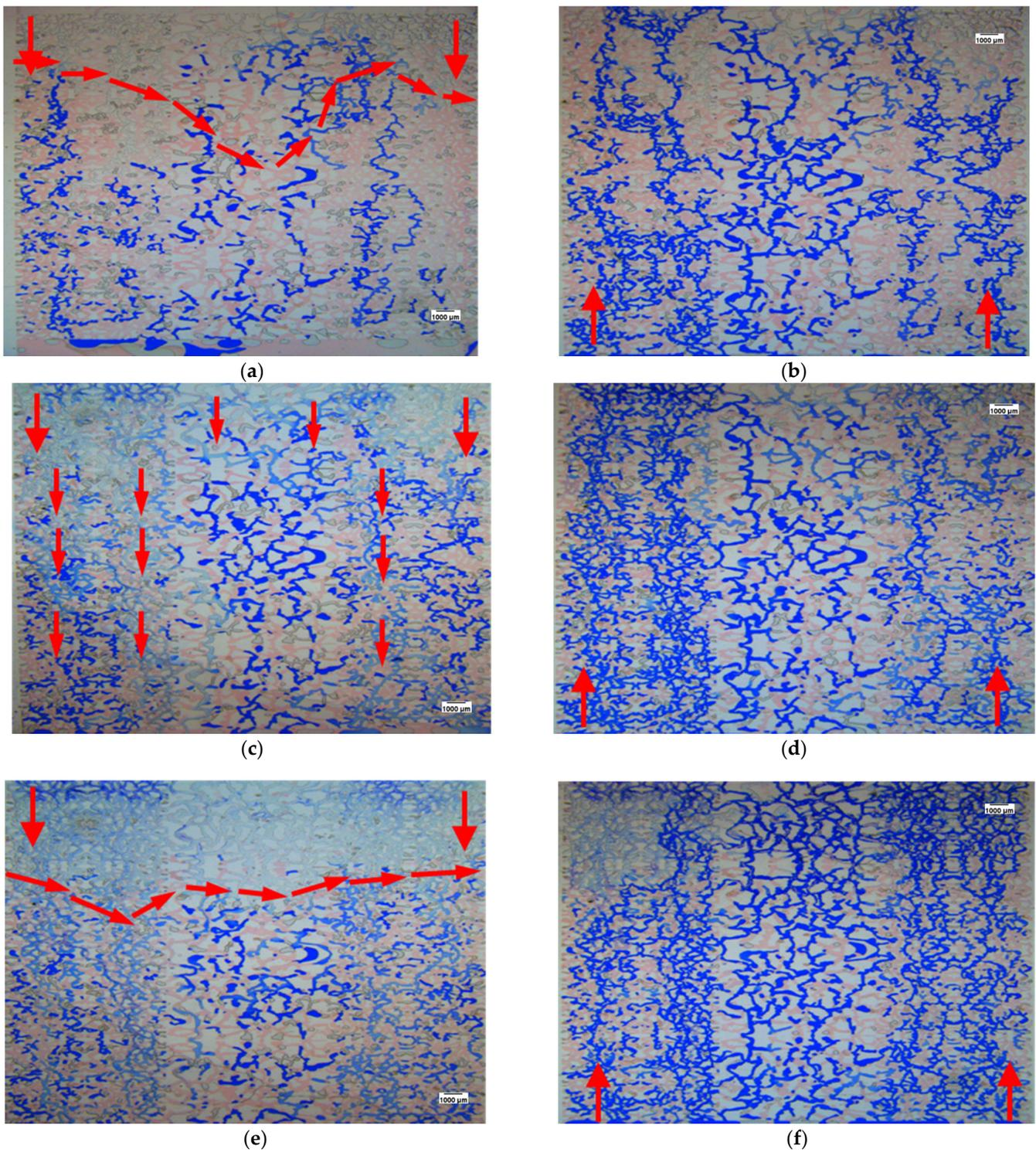
**Figure 15.** The process diagram of the heterogeneous model gel-emulsifier compound water shutoff process. (a) The first gel injection, (b) the second water invasion, (c) the first emulsifier injection, (d) the third water invasion, (e) the second gel injection, (f) the fourth water invasion.
