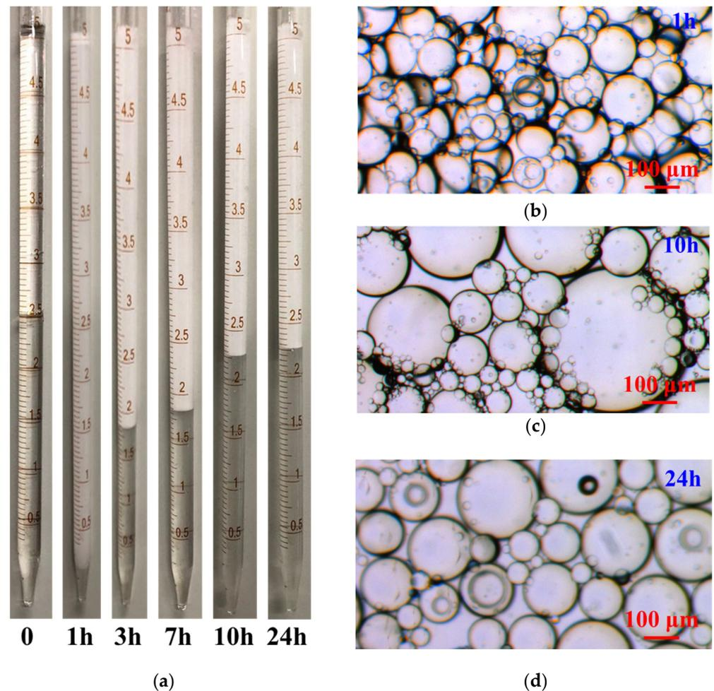
**Figure 2.** Emulsion phase behavior as a function of time at reservoir temperature. (a) Emulsion phase behavior as a function of time at reservoir temperature; (b) the microscopic images of the emulsion at 1 h; (c) the microscopic images of the emulsion at 10 h; (d) the microscopic images of the emulsion at 24 h.
