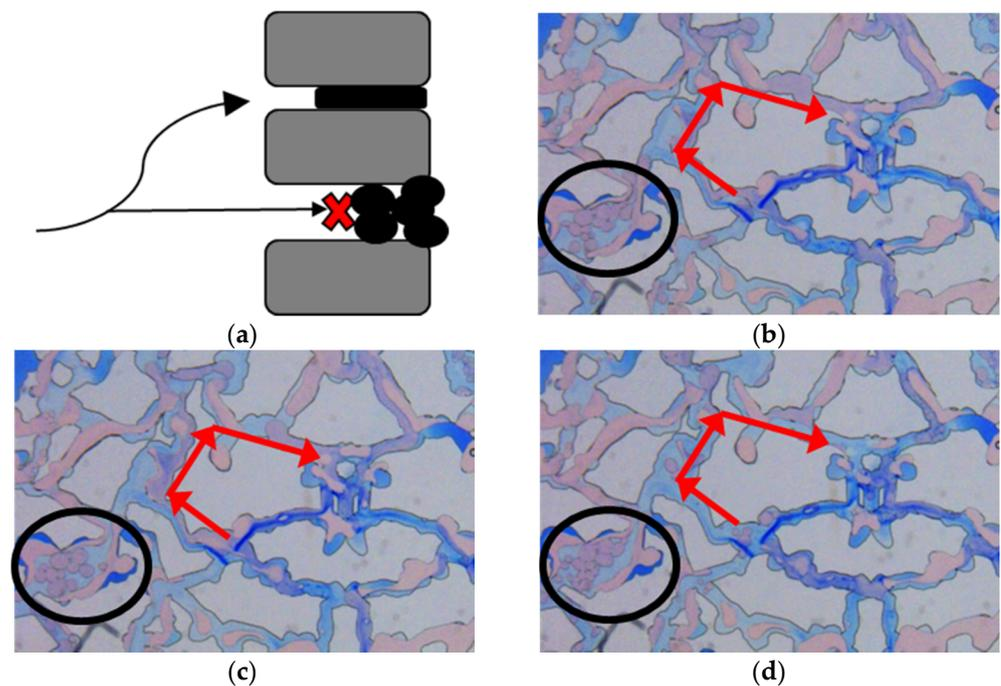
**Figure 8.** Emulsion water plugging mechanism diagram under the action of the emulsifier: (a) the schematic diagram of the emulsion water-plugging mechanism; (b) 0 s; (c) 100 s; (d) 200 s.
