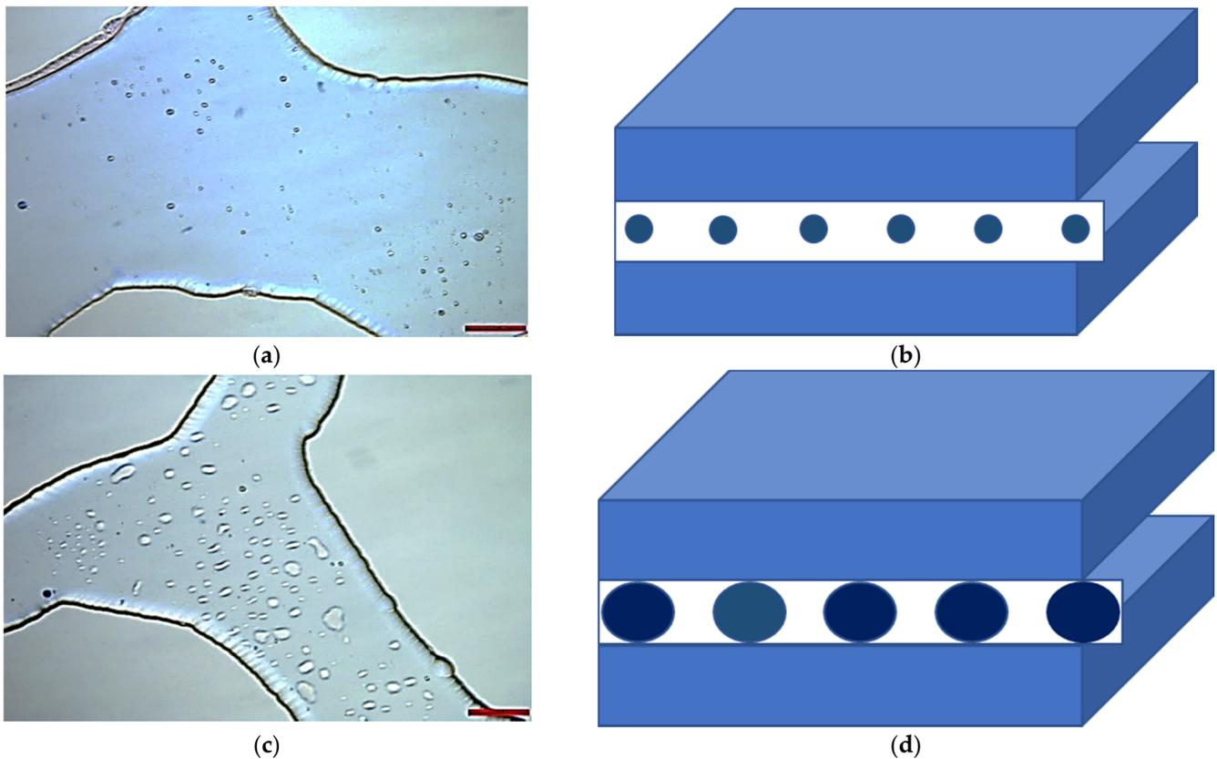
**Figure 11.** Water shutoff mechanism of polymer microspheres. (a) The distribution of polymer microspheres in the channel before expansion; (b) no permeability loss before expansion; (c) the distribution of polymer microspheres in the channel after expansion; (d) permeability loss caused by blocked pores after the expansion of polymer microspheres.
