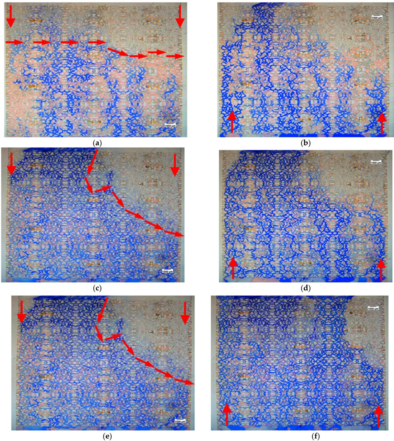
**Figure 14.** The process diagram of the homogeneous model gel-emulsifier compound water shutoff process. (a) The first gel injection, (b) the second water invasion, (c) the first emulsifier injection, (d) the third water invasion, (e) the second gel injection, (f) the fourth water invasion.
