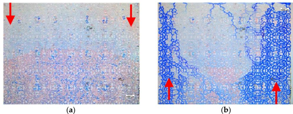
**Figure 12.** Injection of homogeneous model gel system and subsequent water invasion images. (a) The gel is injected along the simulated “horizontal wellbore”; (b) end of the second water flooding.
