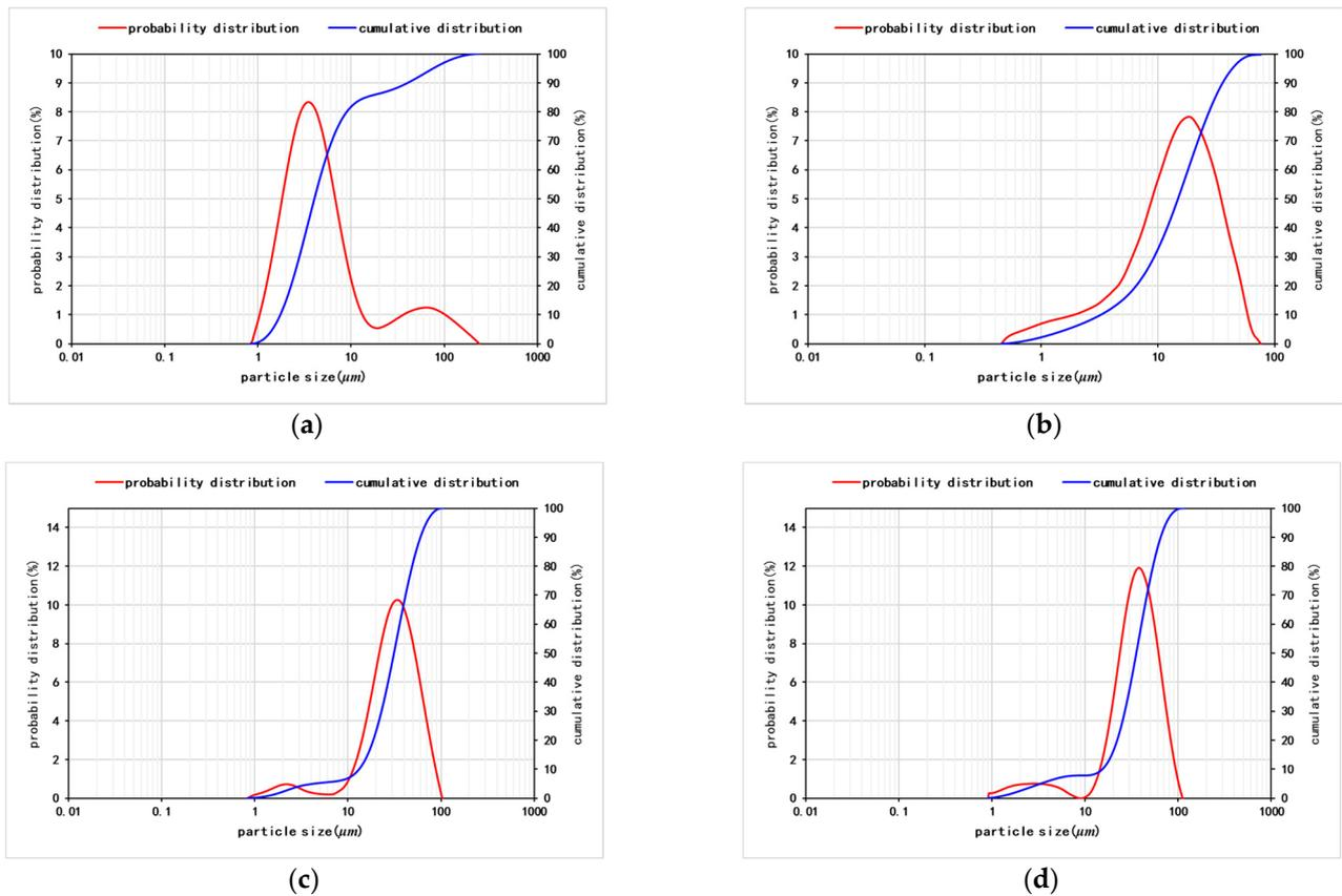
**Figure 3.** The particle size test results of nano-microspheres under different standing times. (a) The newly prepared dispersion on (b) day 1, (c) day 2, and (d) day 3.
