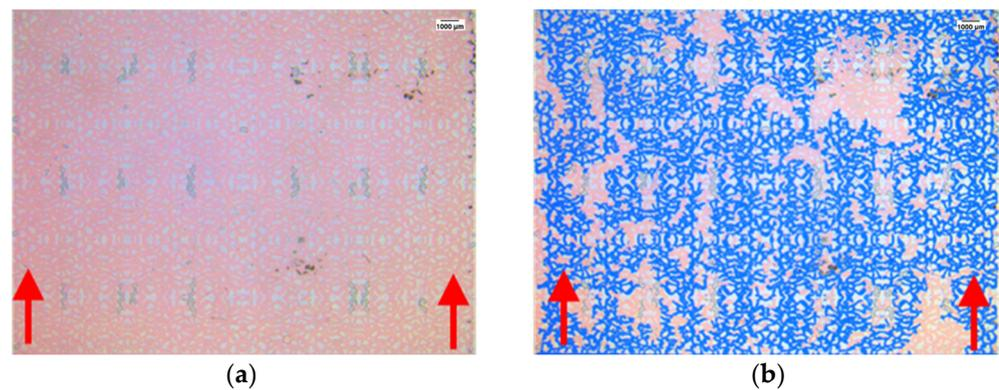
**Figure 5.** The microscopic image of the homogeneous model water flooding process. (a) Saturated oil and (b) end of water flooding.
