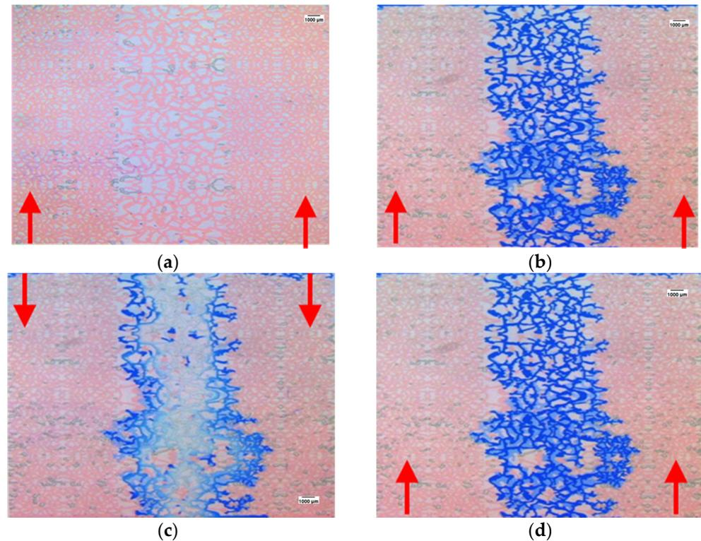
**Figure 7.** Heterogeneous model emulsifier injection and subsequent water invasion images: (a) saturated oil; (b) end of the first water flooding; (c) the emulsifier injected along the simulated “horizontal wellbore”; (d) end of the second water flooding.
