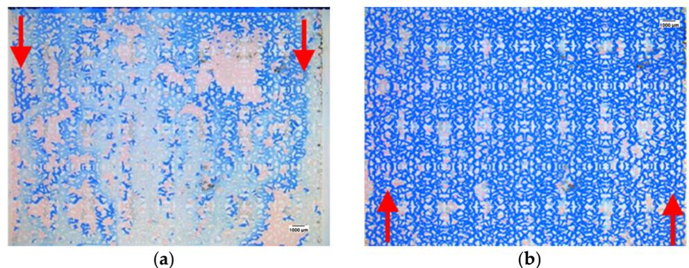
**Figure 6.** Emulsifier injection and subsequent water-invasion images of the homogeneous model: (a) the emulsifier is injected along the simulated “horizontal wellbore” and (b) the end of the second water flooding.
