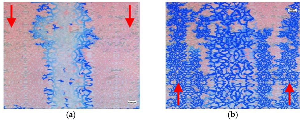
**Figure 10.** The subsequent water invasion process diagram after polymer microsphere injection and microsphere expansion in the heterogeneous model. (a) The emulsifier is injected along the simulated “horizontal wellbore”; (b) end of the second water flooding.
