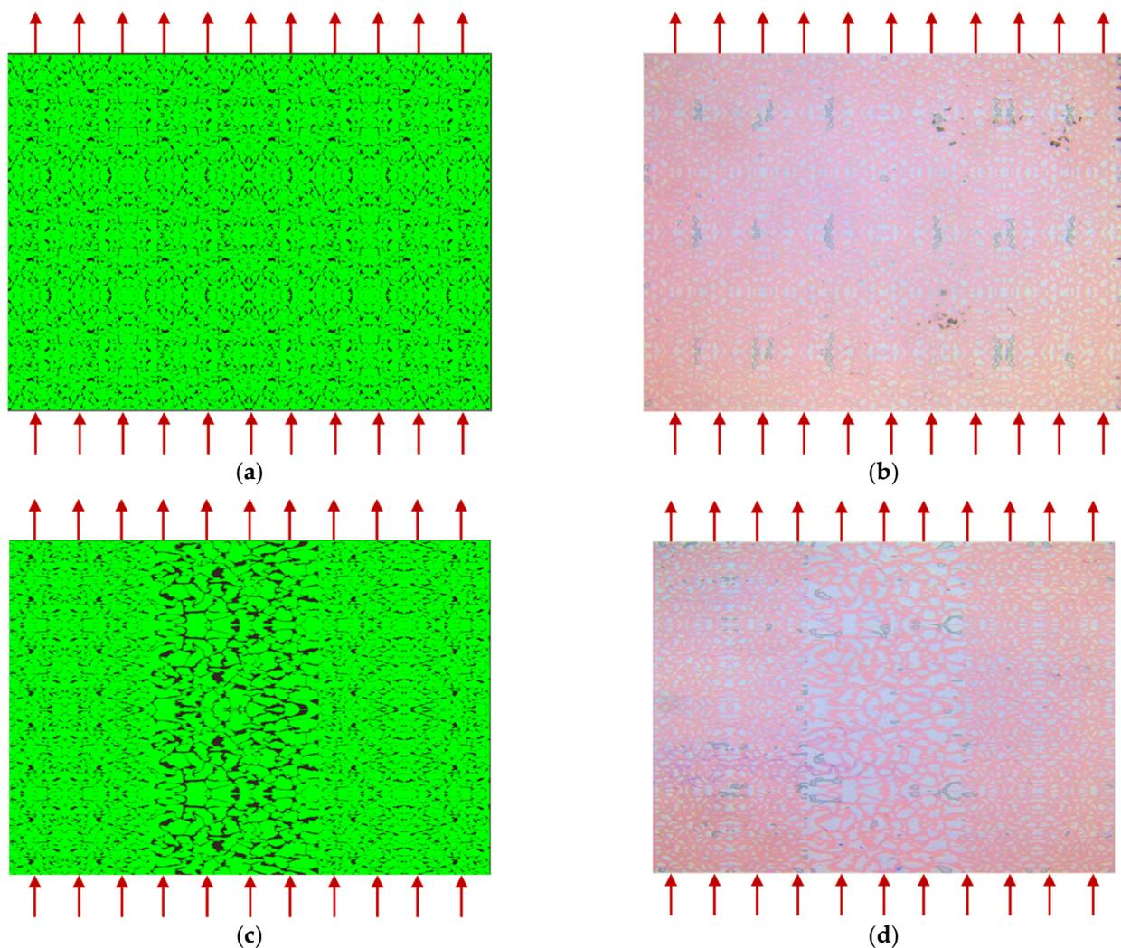
**Figure 1.** Two types of microfluidic models. (a) The schematic diagram of the homogeneous model; (b) the homogeneous model; (c) the schematic diagram of a heterogeneous model; (d) the heterogeneous model.
