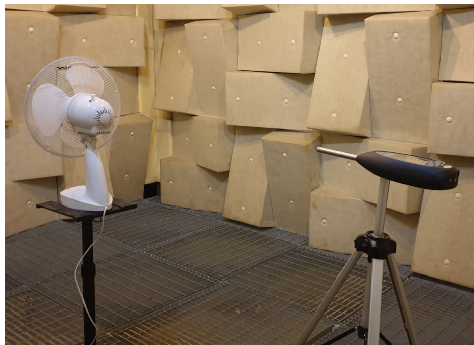
Figure 3. Set up of measurements in an anechoic chamber. The decision to place the sound level meter behind the fan was made to avoid the influence of the air flow on the measurement.
