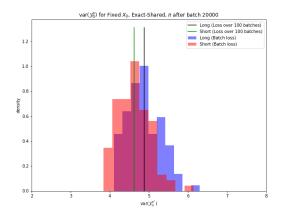
**Figure 8.** Distribution of batch losses for the rollback  $\mathcal{Y}_0^{\pi}$  for the strategies after the 20,000th batch in the optimization. Straddle. Backward method with exact backward step. Single DNN for  $\pi$ . Batch size 512.
