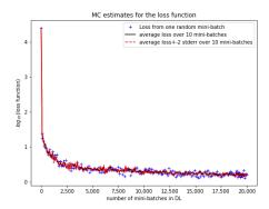
**Figure 2.** Loss function over 20,000 mini-batches for long call combination for batch-variance method with exact backward step. Loss functions for the other variants look very similar. Batch size 512.
