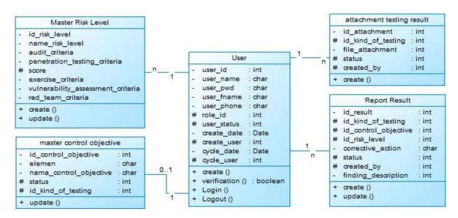
Figure 10. Class Diagram of Risk Treatment Plan Control Test Applications.
