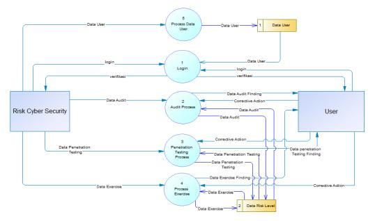
Figure 9. Data Flow Diagram of the Level 1 Testing Using Audit, Exercise and Penetration Testing.
