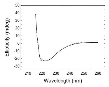
**Figure S2.** Far-UV circular dichroism spectrum of the 3CLpro-rutin complex (continuous line) and addition of individual spectra of 3CLpro and rutin (dashed line), recorded at  $10~\mu M$  protein concentration and  $100~\mu M$  ligand concentration, under the same conditions. The presence of DMSO at low concentration caused degradation of the signal below 215 nm, as reported previously (Abian et al. Int. J. Biol. Macromol. **2020**, *164*, 1693–1703).
