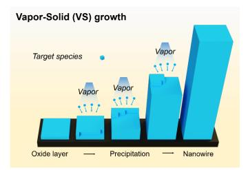
Figure 4. A typical Vapor–Solid (VS) growth mechanism in nanowire fabrication.
