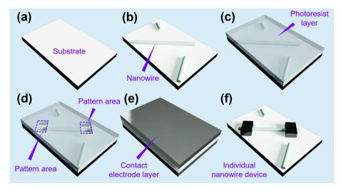
Figure 12. A schematic diagram illustrating the fabrication processes of individual nanowire devices: (a) substrate; (b) transferring nanowires onto the substrate; (c) photoresist coating (sacrificial layer); (d) sacrificial layer patterning; (e) contact electrode deposition; (f) individual nanowire device after lift-off process.
