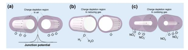
**Figure 24.** A schematic diagram of conventional nanowire–nanowire junction sensors: (**a**) nanowire conducting channel exposed to ambient; (**b**) nanowire conducting channel exposed to oxidization gas; and (**c**) nanowire conducting channel exposed to reducing gas.
