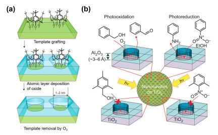
Figure 26. (a) The fabrication process of molecules imprinted oxide; and (b) the preferential reaction with gas species. Reprinted from reference [359] with permission from the Nature publishing group.
