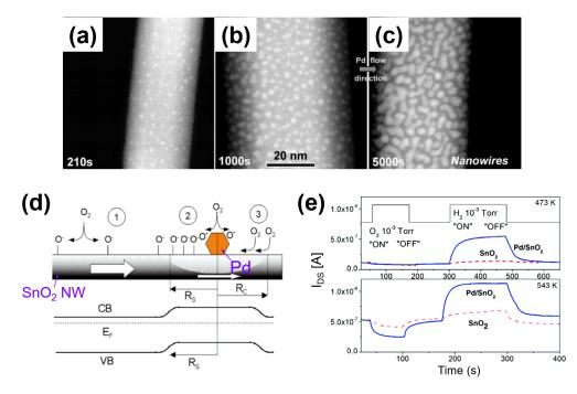
**Figure 18.** (**a**–**c**) Nanoparticles decorated metal–oxide nanowire with different coverage; (**d**) schematic depiction of the three major processes taking place at a  $SnO_2$  nanowire surface and their band diagram; and (**e**) compared studies of the sensing performance of  $SnO_2$  and  $SnO_2/Pd$  nanowire sensor devices. Reprinted from reference [273] with permission from the American Chemical Society.
