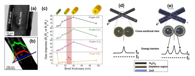
Figure 20. (a) Nanowire with  $SnO_2$  core and ZnO shell structure; (b) EDS of core-shell nanowire; (c) shell thicknessdependent sensing performance towards CO, benzene, toluene, and NO<sub>2</sub>. Reprinted from reference [327] with permission from the American Chemical Society. (d,e) Schematics of the hydrogen-sensing mechanism for  $In_2O_3$  nanowires and  $In_2O_3/ZnO$  C–S nanowires sensors. Reprinted from reference [334] Copyright 2011 Elsevier.
