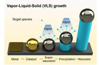
Figure 2. A typical vapor-liquid-solid (VLS) growth mechanism in metal-oxide nanowire fabrication.
