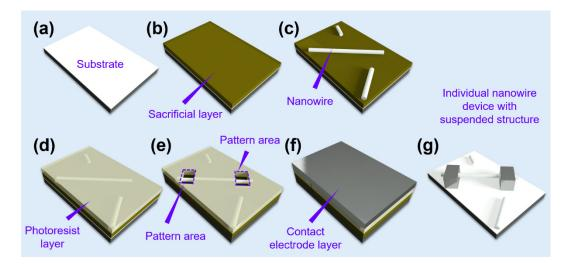
**Figure 13.** A schematic diagram of the individual suspended nanowire device fabrication process: (**a**) substrate; (**b**) photoresist coating (sacrificial layer); (**c**) transferring nanowires onto the substrate; (**d**) photoresist coating (sacrificial layer); (**e**) sacrificial layer patterning; (**f**) contact electrode deposition; and (**g**) individual nanowire device with suspended structure after the lift-off process.
