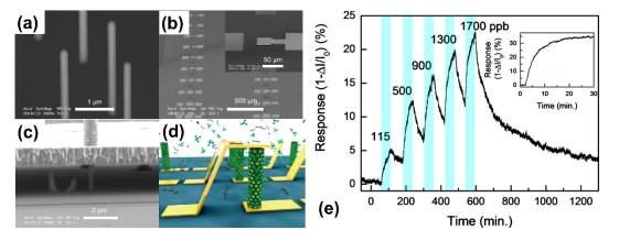
**Figure 14.** The fabrication process of the individual vertical nanowire device: (**a**) as-grown nanowires; (**b**) patterned nanowire arrays with air bridging contact; (**c**) a side view of an air bridge contact; (**d**) schematic image of the individual nanowire with a vertical structure; (**e**) the gas sensing performance of vertical aligned indium arsenide (InAs) nanowires sensor. Reprinted from reference [223] with permission from the American Chemical Society.
