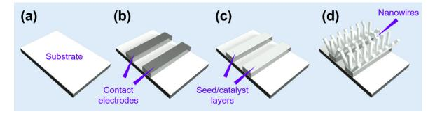
**Figure 16.** A typical method for making bridging metal–oxide nanowires device: (a) substrate; (b) bottom electrode deposition; (c) seed/catalyst layer deposition; and (d) in situ growth of metal–oxide nanowire on electrodes.
