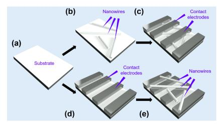
**Figure 15.** Two typical methods for making a mat-like metal–oxide nanowires device: (**a**) platform; (**b**) nanowires transferred onto the platform; (**c**) contact electrode deposition; (**d**) contact electrode deposition; and (**e**) nanowires transferred onto the platform.
