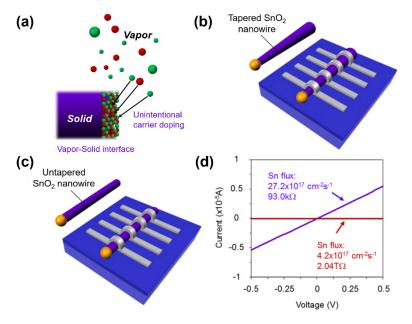
**Figure 5.** Anomalous electrical properties of VS growth nanowire: (**a**) a schematic image of unintentional carrier doping occurs at the vapor–solid interface during VS growth; (**b**) single tapered VS+VLS growth SnO<sub>2</sub> nanowire device; (**c**) single untapered VLS growth SnO<sub>2</sub> nanowire device; (**d**) IV curves of VS growth (93.0 k $\Omega$ ) and VLS growth nanowire (2.04 T $\Omega$ ); Reprinted from reference [79] with permission from the American Chemical Society.
