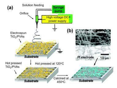
**Figure 10.** (a) Schematic diagram of the processing steps used to fabricate  $TiO_2$  nanofiber mats on  $Al_2O_3$  substrates with interdigitated Pt electrode arrays. PVA (Polyvinyl acetate); and (b) the micrograph of a calcined TiO2 nanofiber mat on top of the  $Al_2O_3$  substrate (dark region) and Pt electrode (bright region). Reprinted from reference [201] with permission from the American Chemical Society.
