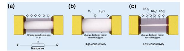
**Figure 22.** A schematic diagram of conventional chemiresistor sensors: (**a**) nanowire conducting channel exposed to ambient; (**b**) nanowire conducting channel exposed to reducing gases; and (**c**) nanowire conducting channel exposed to oxidizing gases.
