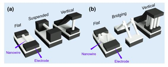
**Figure 11.** Schematic image of (**a**) an individual nanowire device with different structures (flat, suspended, and vertical); and (**b**) multiple nanowire device (flat, bridging, and vertical).
