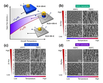
**Figure 3.** (a) The concept of "materials flux window" for nanowire growth (VLS, Vapor–Liquid–Solid; VS, Vapor–Solid); SEM image of (b) SnO<sub>2</sub> nanowires; (c) ZnO nanowires; and (d) MgO nanowires fabricated under the guidance of 'materials flux window'. Reprinted from reference [83] with permission from the American Chemical Society.
