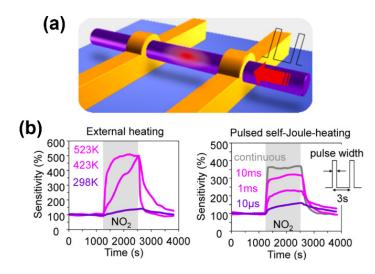
**Figure 28.** (a) Suspended nanowire device; and (b) comparison between the conventional external heating device and pulsed self-joule-heating device. Reprinted from reference [220] with permission from the American Chemical Society.
