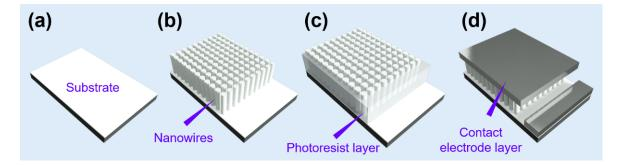
**Figure 17.** A typical method for making a vertical metal–oxide nanowires device: (**a**) the substrate with the seed/catalyst layer; (**b**) nanowires are grown vertically; (**c**) photoresist coating with the further etching process; and (**d**) top contact electrode deposition and the removal of photoresist.
