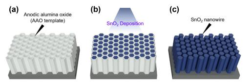
**Figure 8.** Schematic image of (**a**) the highly regular AAO template; (**b**) the template cross-section with nanowires deposited inside the nanopores; and (**c**) nanowires after removing the AAO template.
