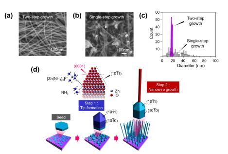
**Figure 25.** (a) SEM image of two-step growth ZnO nanowire; (b) SEM image of conventional single-step growth ZnO nanowire; (c) comparison of ZnO nanowire diameter distribution grown by single-step and two-step method; (d) the mechanism of the synthesis of monodispersed sized ZnO nanowires from randomly sized seeds. Reprinted from reference [355] with permission from the American Chemical Society.
