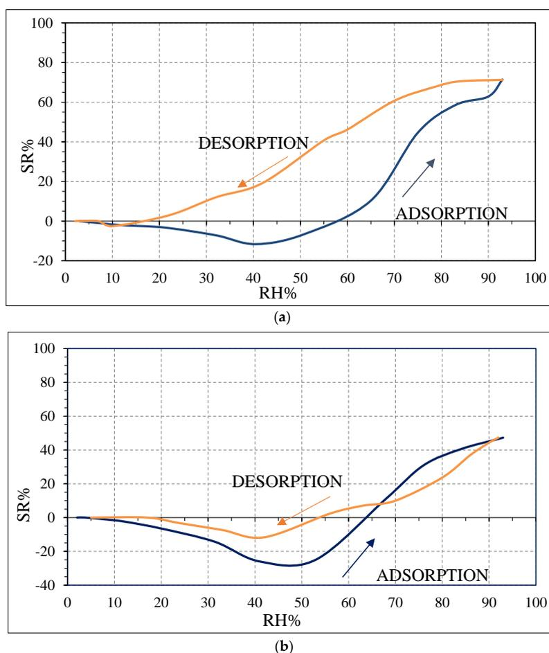
**Figure 12.** Sensor response toward relative humidity for SWP700 biochar with (a) 10%; (b) 20% of PVP acting as polymeric binder.
