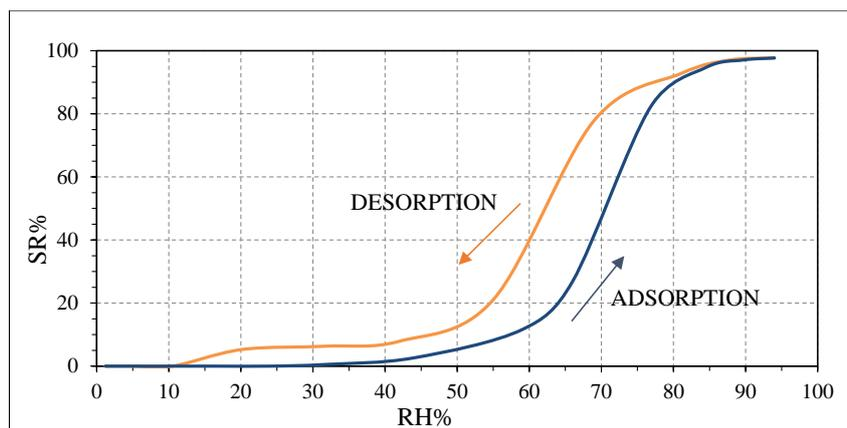
**Figure 11.** Polyvinylpyrrolidone (PVP) sensor response toward relative humidity.
