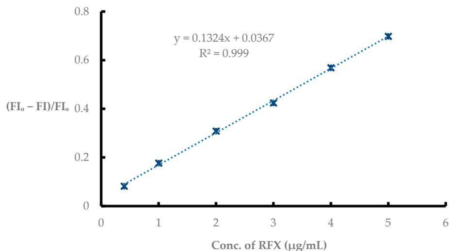
**Figure 5.** Construction of the calibration curve for the determination of RFX by the proposed spectrofluorimetric method.
