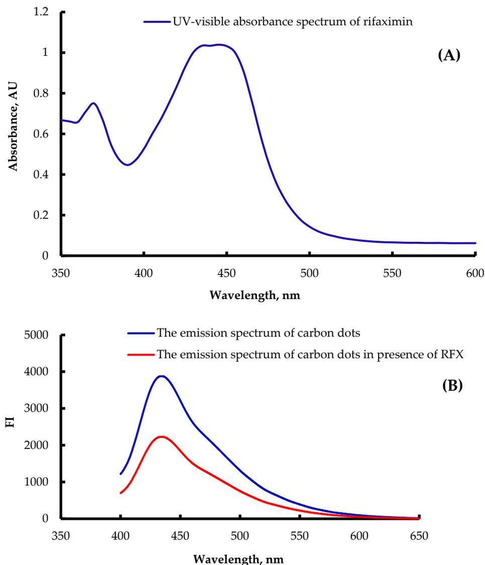
**Figure 3.** (A) For the absorbance spectrum for rifaximin and (B) for quenching the fluorescence emission spectrum of the produced carbon dots by rifaximin.
