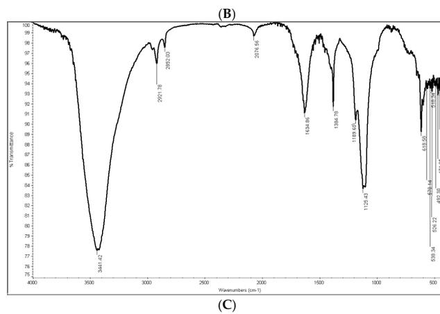
**Figure 2.** Characterization of the produced carbon dots: (A) for TEM; (B) for excitation and emission fluorescence spectra, (C) for FTIR spectrum.
