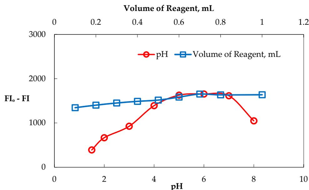
**Figure 4.** Effect of pH and volume of the reagent on the quenching of the fluorescence intensity of the prepared carbon dots for determining RFX (3.0 µg/mL).
