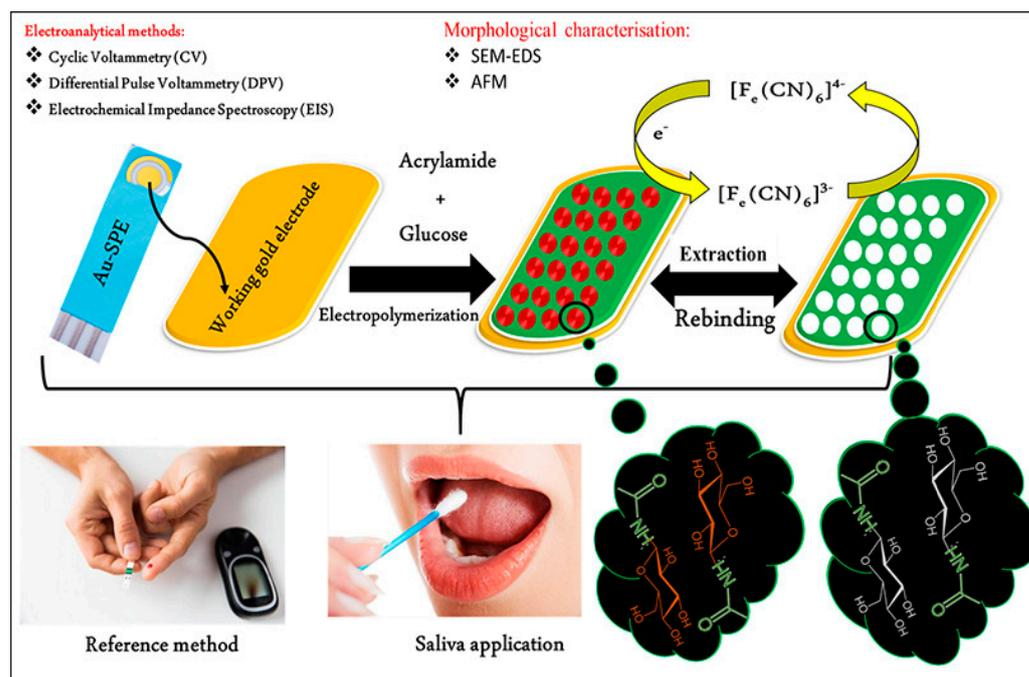
**Figure 4.** Fabrication of a MIP-based Au SPE by electropolymerizing AAM/NNMBA in the presence of glucose and its application in saliva samples. Figure reproduced with permission from ref. [86]. Copyright 2019, Elsevier.
