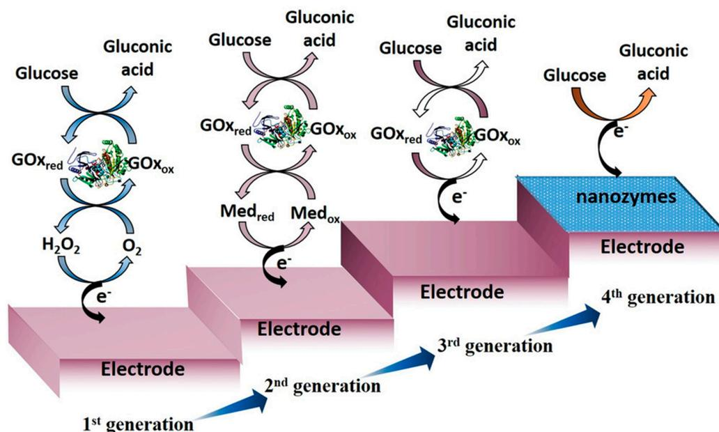
**Figure 1.** Schematic representation of the working principle of different generations of electrochemical glucose sensors. Figure reproduced with permission from ref. [16].
