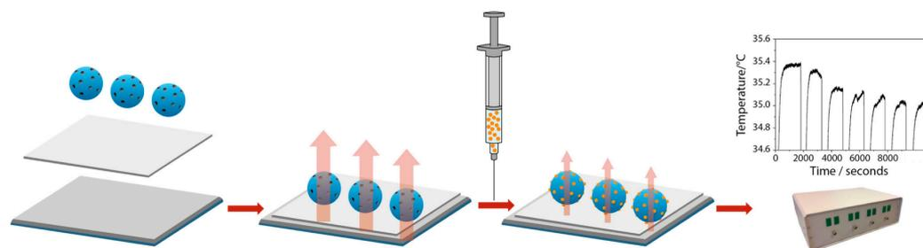
**Figure 8.** Representation of HTM analysis after glucose rebinding to the MIP-based platform. Figure reproduced with permission from ref. [87].
