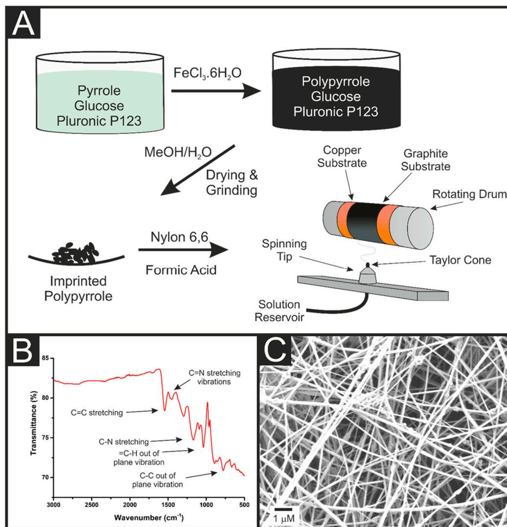
**Figure 5.** (A) Illustration of the production of electrospun MIP sensors. (B) FT–IR analysis of the polypyrrole MIP. (C) Image of electrospun nylon fibers embedded with PPy MIPs for the detection of glucose. Figure reproduced with permission from ref. [77]. Copyright 2021, American Chemical Society.
