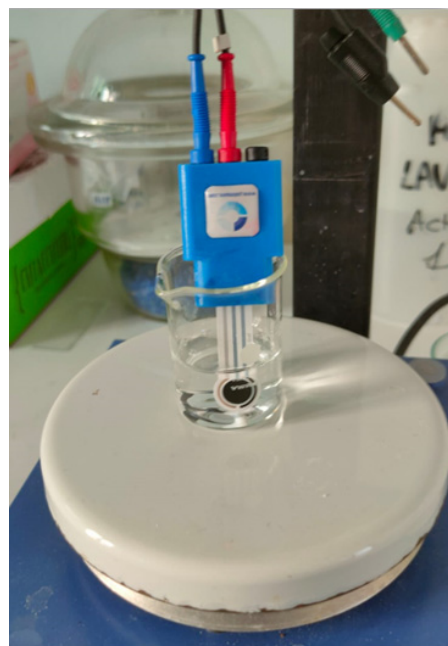
Figure S2. Picture of the experimental setup for potentiometric and electrochemical impedance spectroscopy (EIS) measurements.
