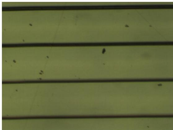
**Figure 5.** Polarisation microscopic photos of channel waveguides using a microbeam of 11 MeV  $C^{4+}$  ions at fluences of  $2, 1.4, 1.4$  and  $0.46 \cdot 10^{15}$  ions/cm<sup>2</sup> (from top to bottom). Width of the channel waveguides is 15  $\mu\text{m}$ .
