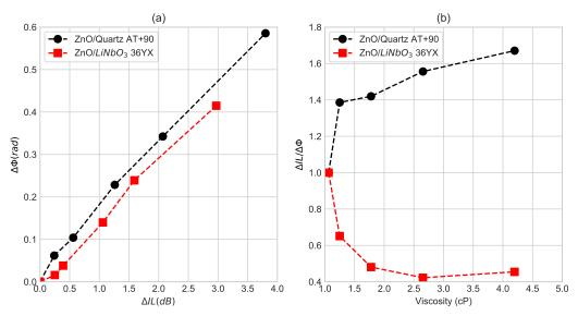
**Figure 4.** Experimental phase shift vs. insertion loss for different fluid viscosity (a) and relative acoustic ratio as a function of the viscosity (b) for both structures.
