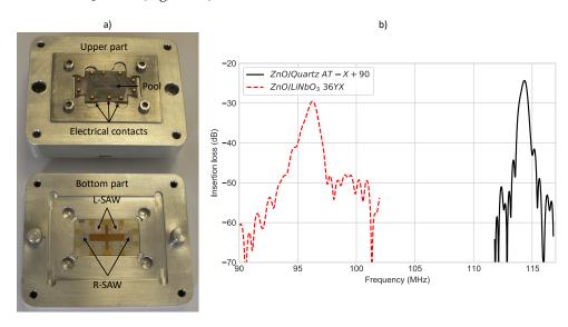
**Figure 3.** Microfluidic cell and  $ZnO/Quartz\ AT - X + 90$  structure (a); insertion loss of the transmission response (S21) observed with fluid (water) interaction for both L-SAW devices (b).
