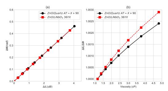
**Figure 5.** Theoretical phase shift vs. insertion loss for different fluid viscosity [0.9 cP - 4.2 cP] (a) and relative acoustic ratio as a function of the viscosity (b) for both structures.
