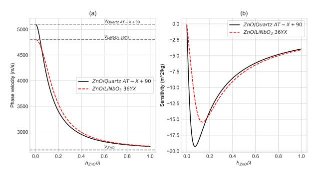
**Figure 2.** Theoretical calculated phase velocity (**a**) and mass sensitivity (**b**) for the first Love mode as a function of normalized guiding-layer thickness.
