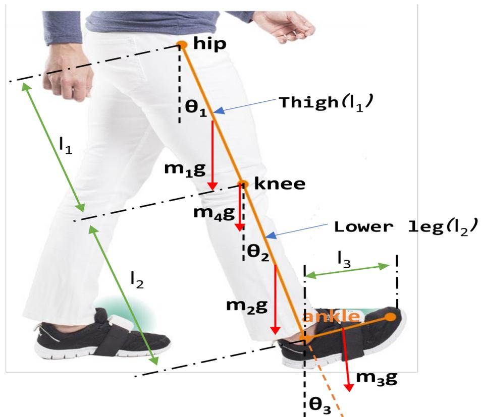
Figure 6. Force balance diagram of the lower leg.
