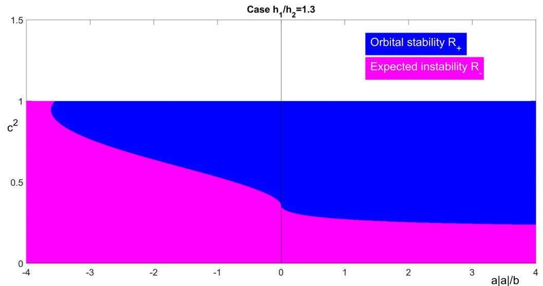
Figure 1. The region of orbital stability ( $d'' > 0$ ) for  $h_1/h_2 = 1.3, \frac{a|a|}{b} \in (-4,4)$  and  $c^2 \in (0,1)$ : left half-plane is for  $a < 0$ ; right half-plane is for  $a > 0$ .
