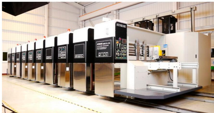
**Figure 3.** High-capacity fixed-type corrugated box precision printing machine (CBPPM) (<http://www.sunrisemachinery.com>).
